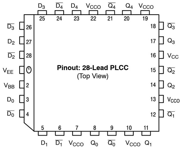
\* All V<sub>CC</sub> and V<sub>CCO</sub> pins are tied together on the die.
