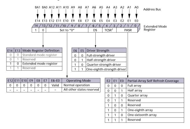
Notes: 1. On-die temperature sensor is used in place of TCSR. Setting these bits will have no effect.
