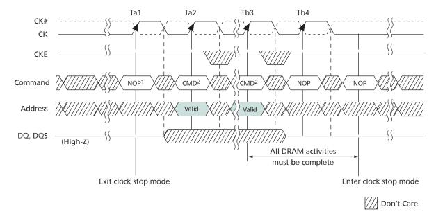
Notes: 1. Prior to Ta1, the device is in clock stop mode. To exit, at least one NOP is required before any valid command is issued.
