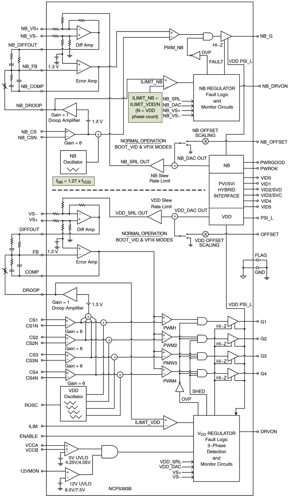
Figure 2. NCP6251 Block Diagram
