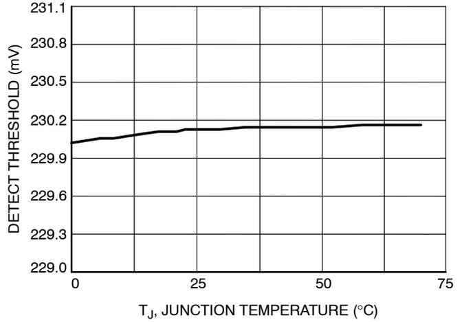
Figure 4. 2/3/4 Phase Detection Threshold vs. Temperature
