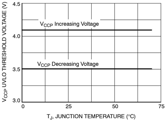
Figure 5. V<sub>CCP</sub> Undervoltage Lockout Threshold Voltage vs. Temperature
