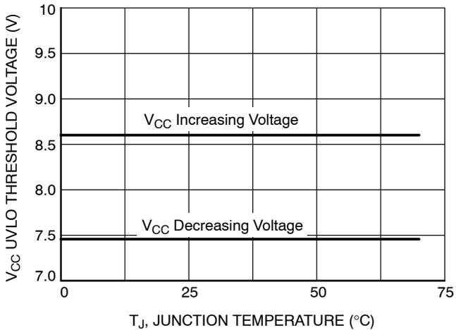
Figure 7. 12VMON Undervoltage Lockout Threshold Voltage vs. Temperature
