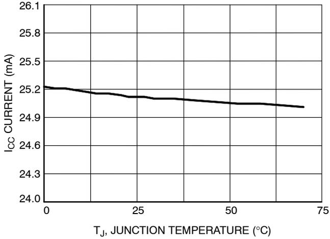
Figure 3. I<sub>CC</sub> Current vs. Temperature
