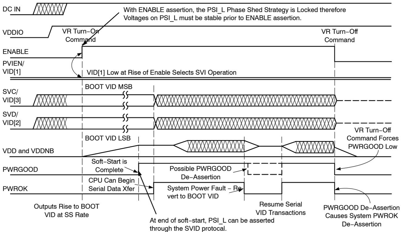
**Figure 10. Power-Up Sequence in Serial Mode Operation**
