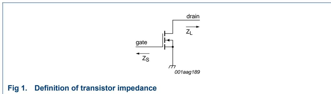
Fig 1. Definition of transistor impedance
