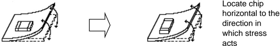
[Chip Mounting Close to Board Separation Point]
