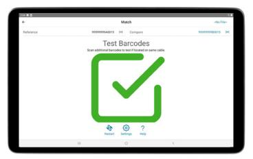
The mobile app **matches** the opposite end of a scanned cable. The software offers notifications when the right end is found, which expedites a tedious process to free up network engineers for more rewarding initiatives.
