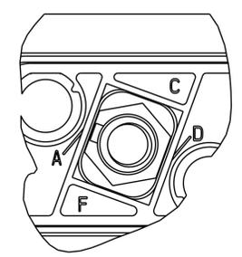
MARKING ON INTERFACIAL SEAL WILL ONLY SHOW A, C, D AND F (CODE A SHOWN FOR REFERENCE)
