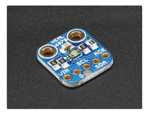
This little sensor is a great way to add UV light sensing to any microcontroller project. The VEML6070 from Vishay has a true UV A light sensor and an I2C-controlled ADC that will take readings and integrate them for you over ~60ms to 500ms.
