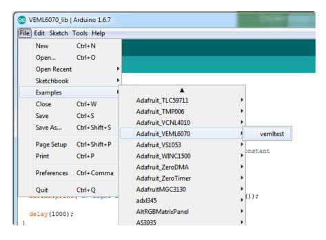
Upload to the Arduino and open up the serial console at 9600 baud to see the UV data output. Note that this is not UV index, its just UV light intensity!
