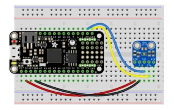
Board 3V to sensor VIN Board GND to sensor G Board SCL to sensor SCL Board SDA to sensor SDA
