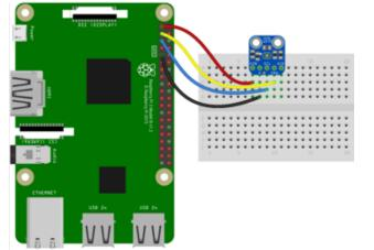
Pi 3V3 to sensor VIN Pi GND to sensor GND
