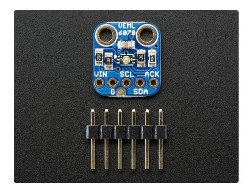
This UV sensor works great with 3 or 5V power or logic, its nice and compact, and its easy to use with any I2C-capable microcontroller.
