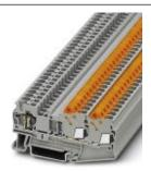
Feed-through terminal block, Connection type: Quick connection, Spring-cage connection, Cross section: 0.5 mm² - 2.5 mm², AWG :20- 14, Width: 6.2 mm, Color: gray, Mounting: NS 35/7,5, NS 35/15
