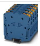
High-current terminal block, Connection method: Power-Turn connection, Cross section: 10 mm<sup>2</sup> - 70 mm<sup>2</sup>, AWG: 8 - 2/0, Width: 20 mm, Color: blue, Mounting type: NS 35/15
