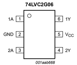
**Fig. 4. Pin configuration SOT363-2 (TSSOP6) and SOT457 (SC-74; TSOP6)**
