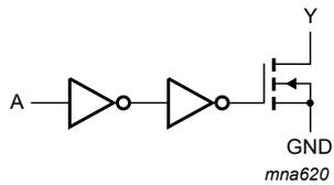
**Fig. 3. Logic diagram (one inverter)**
