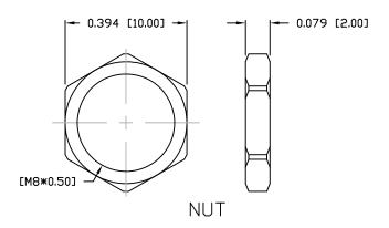
NOTE: MATERIAL HOUSING: PBT UL94V-0, BLACK CONTACT: BRASS SHELL BRASS NUT: BRASS □-RING: EPDM, BLACK FINISH: CONTACT: GOLD PLATED **DVER 50u" NICKEL** SHELL: NICKEL NUT: **NICKEL ELECTRICAL** RATED CURRENT: 1.5A RATED VOLTAGE: 30V INSULATION RESISTANCE: 100 MOhms MIN. CONTACT RESISTANCE: 10 mOhms MAX. IP67 WATER PROOF: **ENVIRONMENT**
