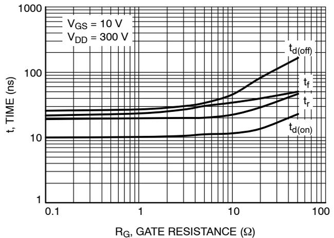
**Figure 12. Resistive Switching Time Variation vs. Gate Resistance**
