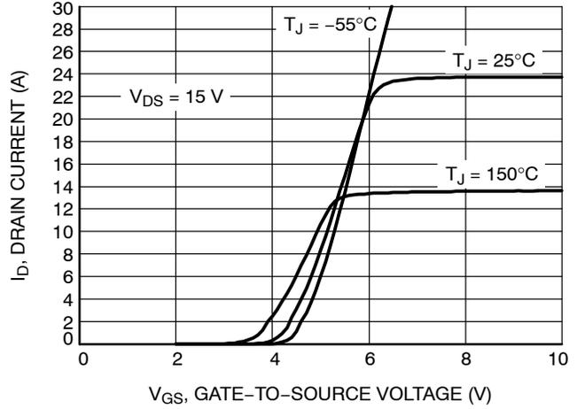
Figure 2. Transfer Characteristics
