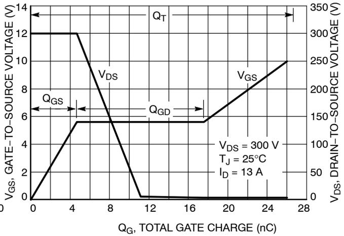
**Figure 10. Gate-to-Source and Drain-to-Source Voltage vs. Total Charge**
