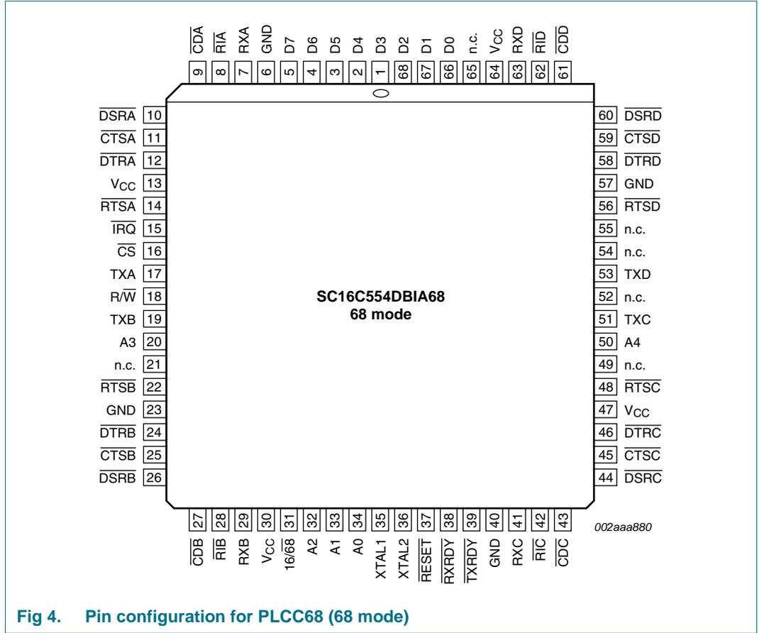
**Fig 4. Pin configuration for PLCC68 (68 mode)**
