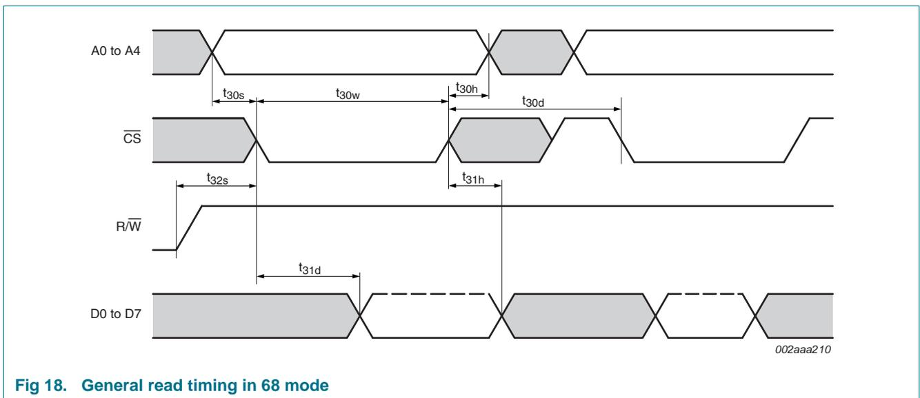
**Fig 18. General read timing in 68 mode**
