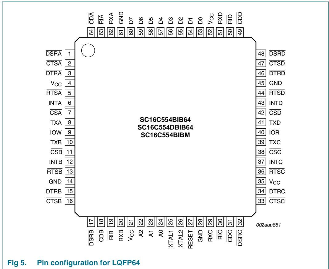
Fig 5. Pin configuration for LQFP64
