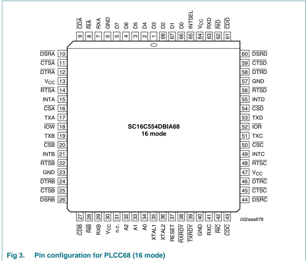
Fig 3. Pin configuration for PLCC68 (16 mode)
