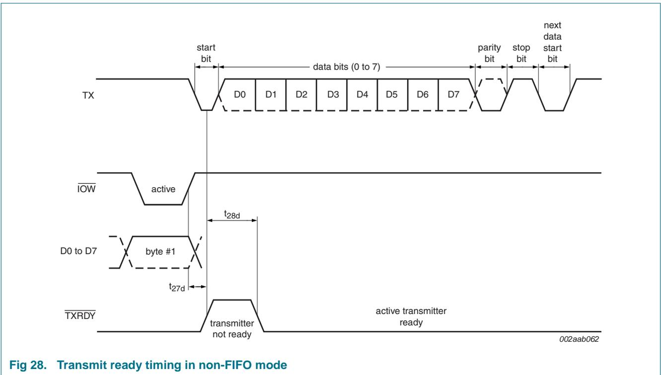
Fig 28. Transmit ready timing in non-FIFO mode
