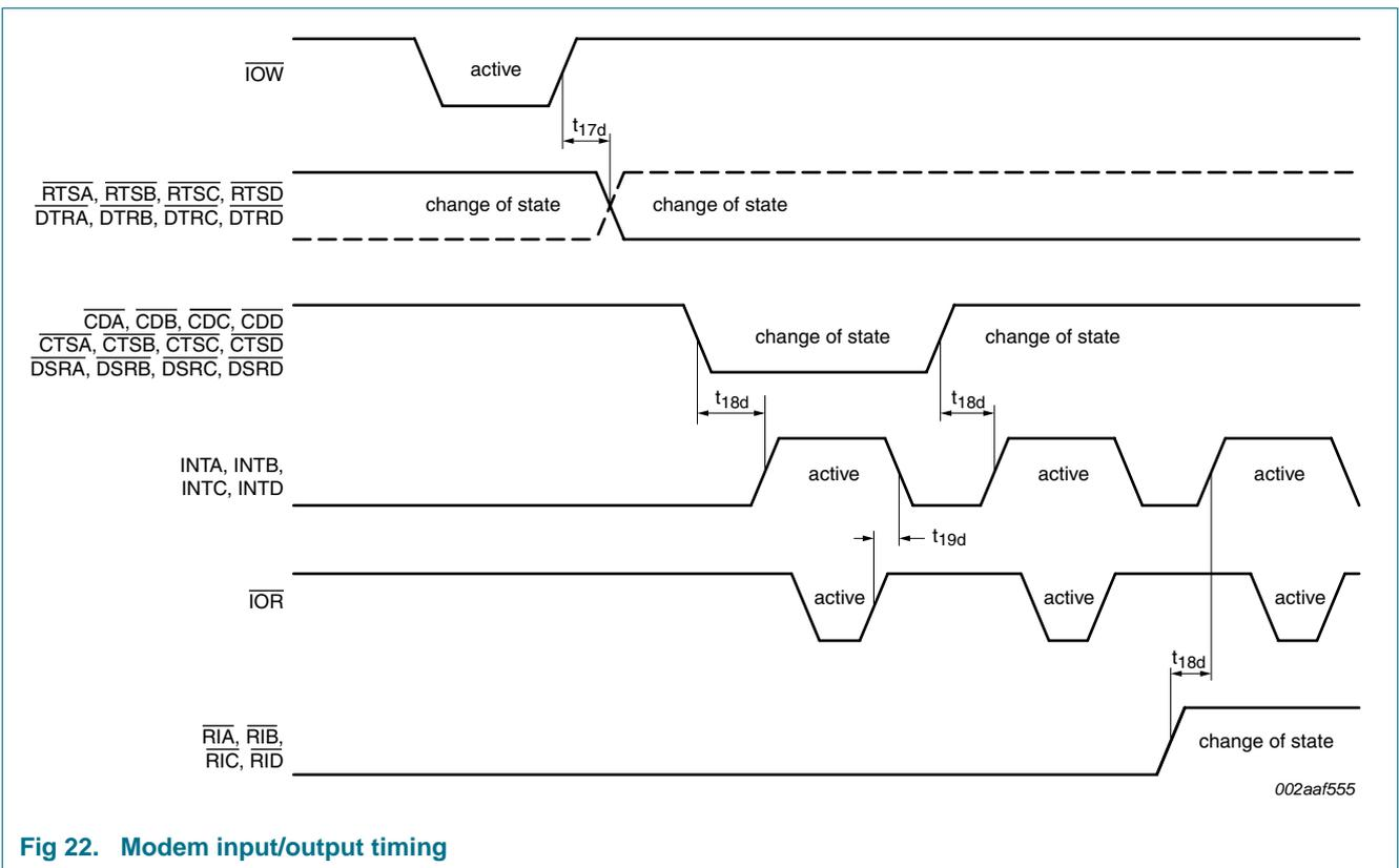
Fig 22. Modem input/output timing
