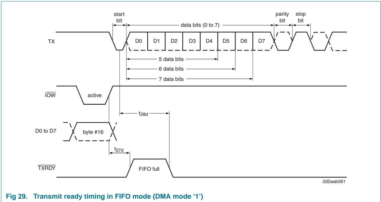
Fig 29. Transmit ready timing in FIFO mode (DMA mode '1')
