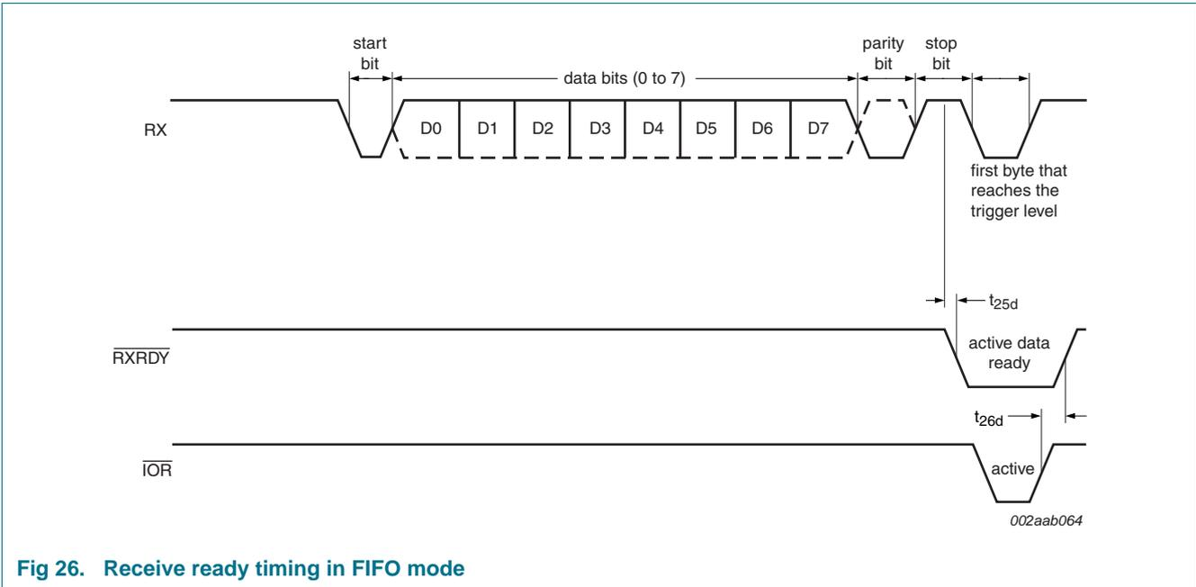
Fig 26. Receive ready timing in FIFO mode
