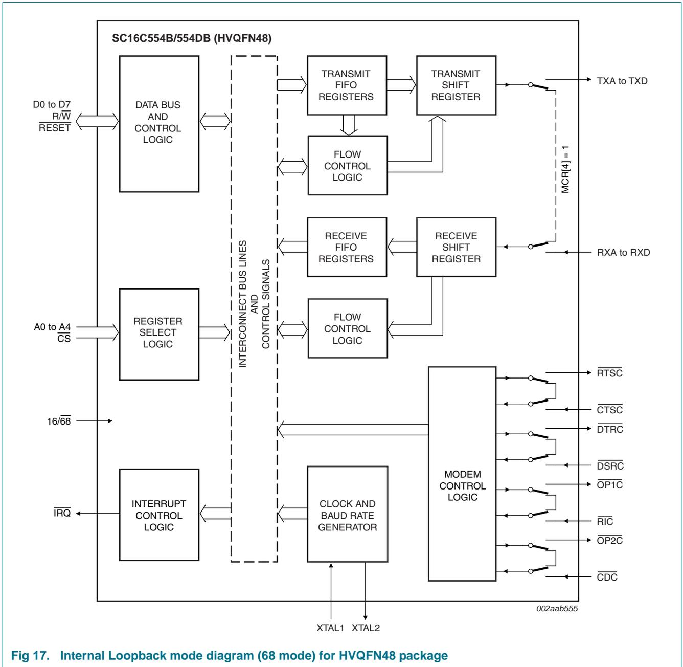
Fig 17. Internal Loopback mode diagram (68 mode) for HVQFN48 package
