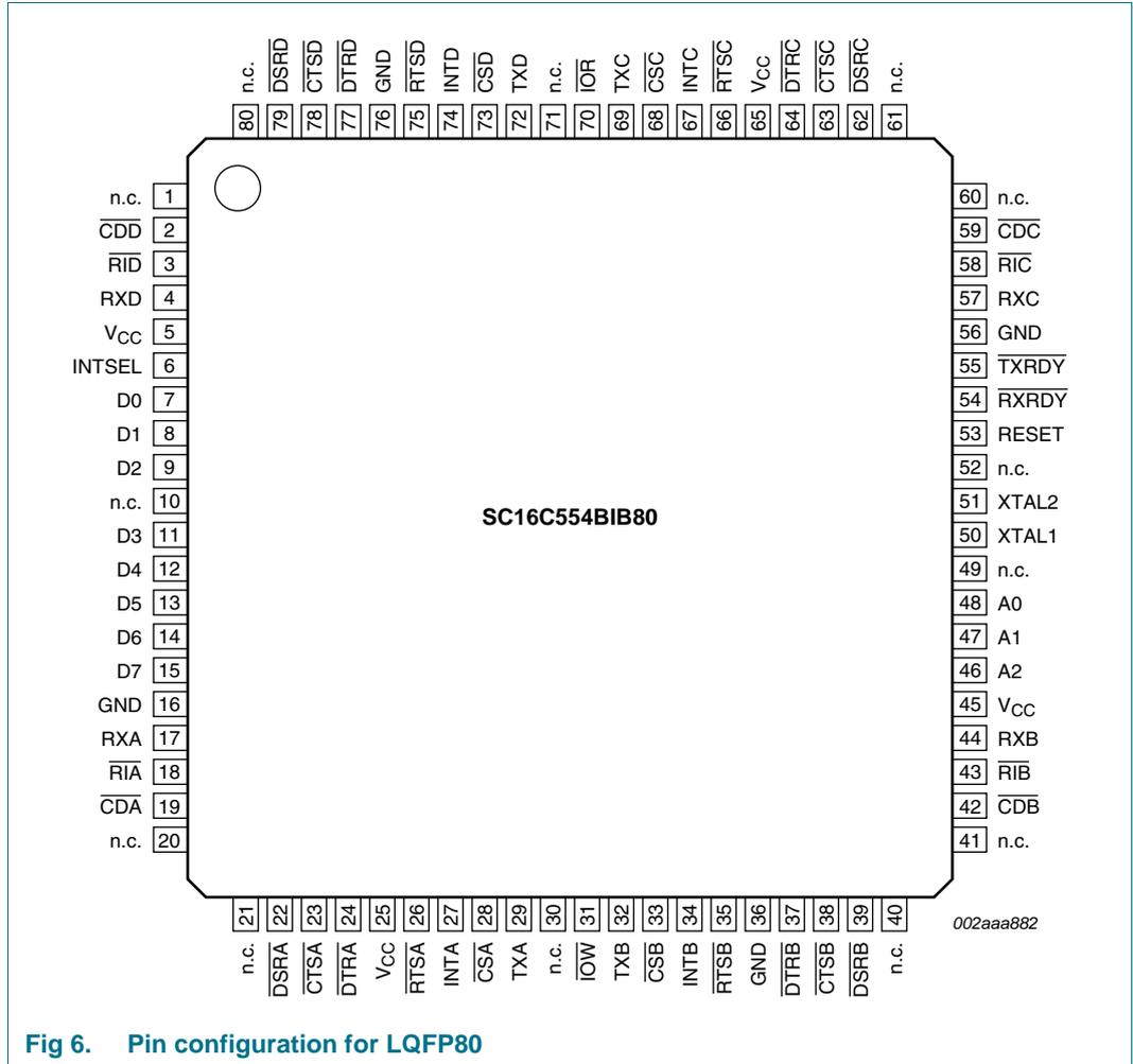
Fig 6. Pin configuration for LQFP80
