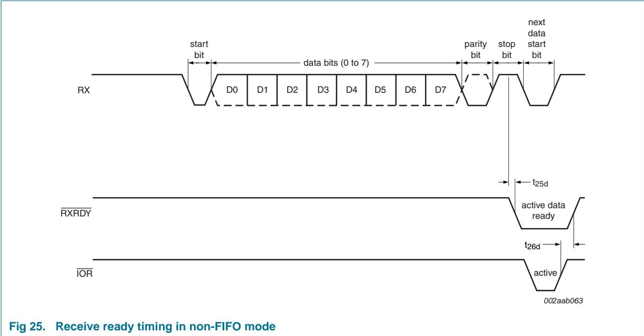
Fig 25. Receive ready timing in non-FIFO mode
