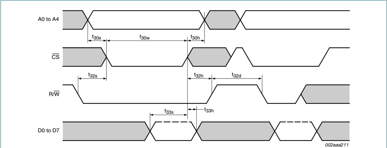
Fig 19. General write timing in 68 mode
