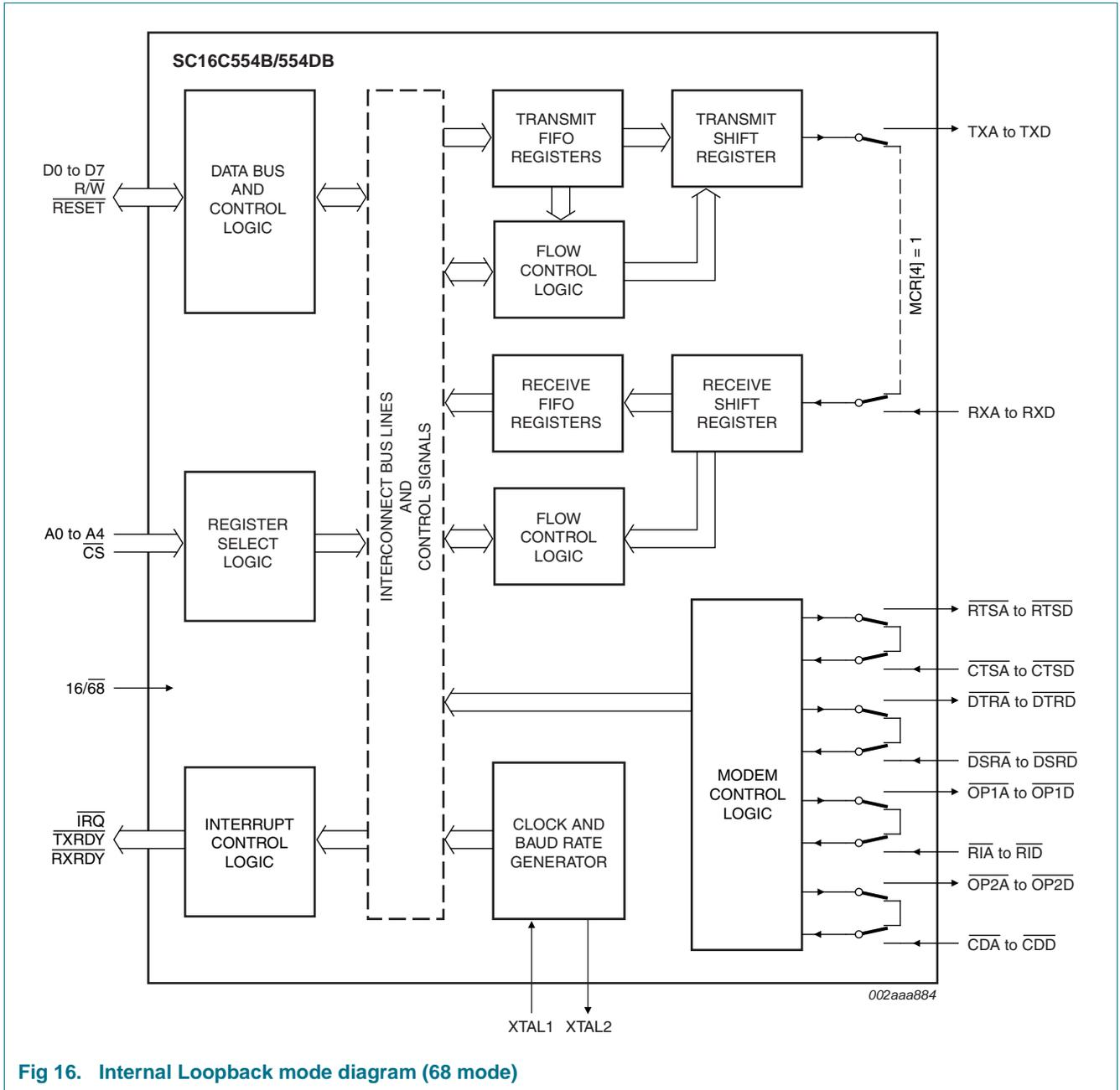
Fig 16. Internal Loopback mode diagram (68 mode)
