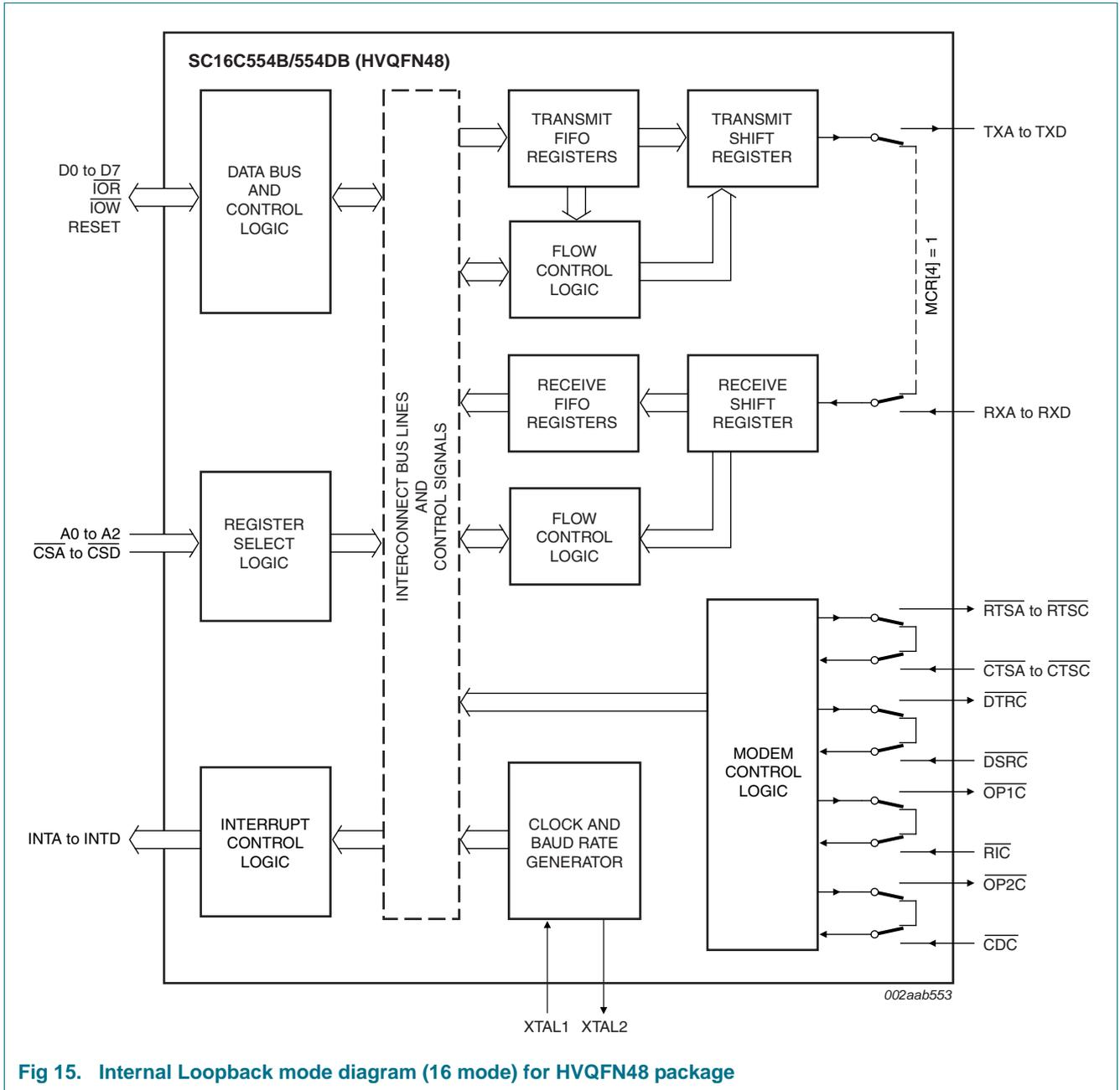
Fig 15. Internal Loopback mode diagram (16 mode) for HVQFN48 package
