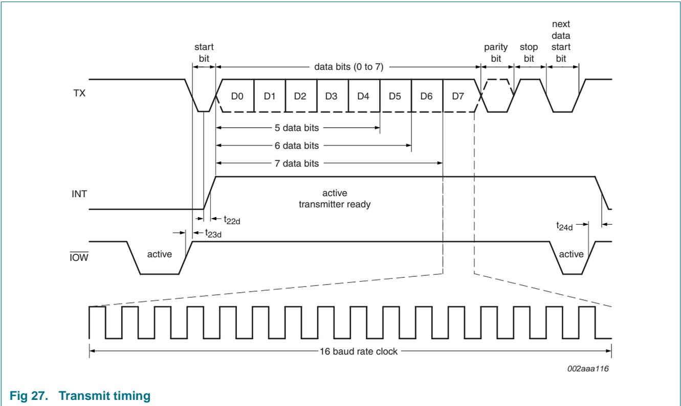
Fig 27. Transmit timing
