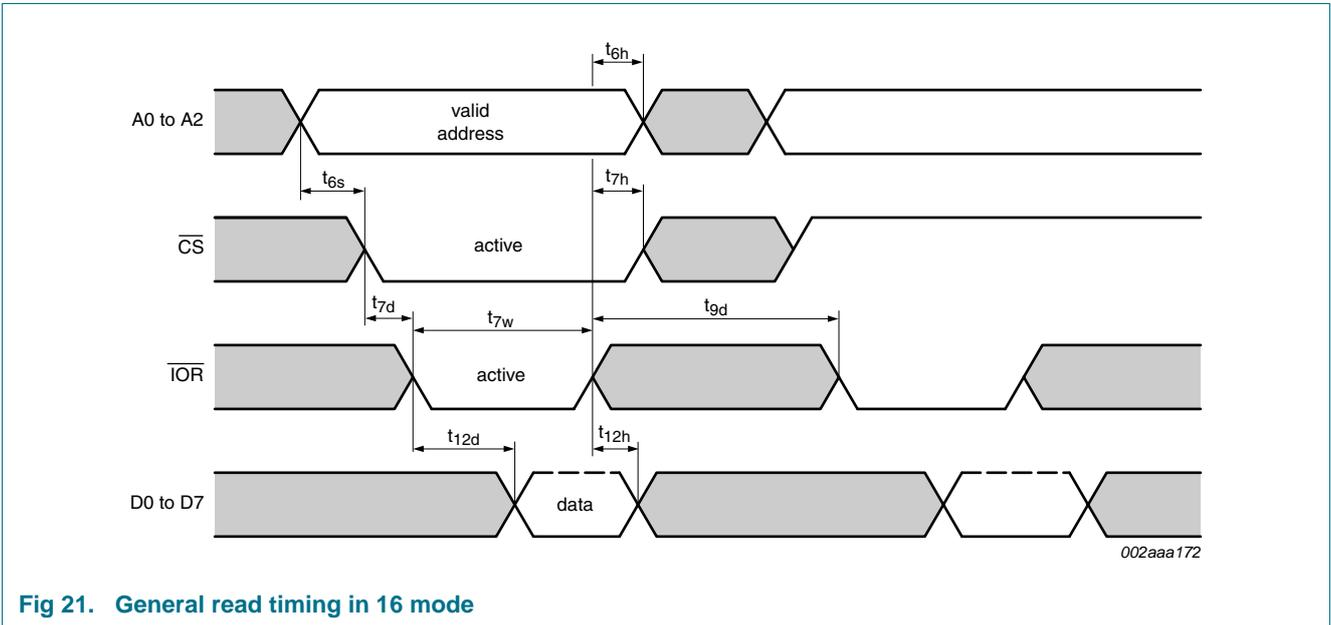
Fig 21. General read timing in 16 mode
