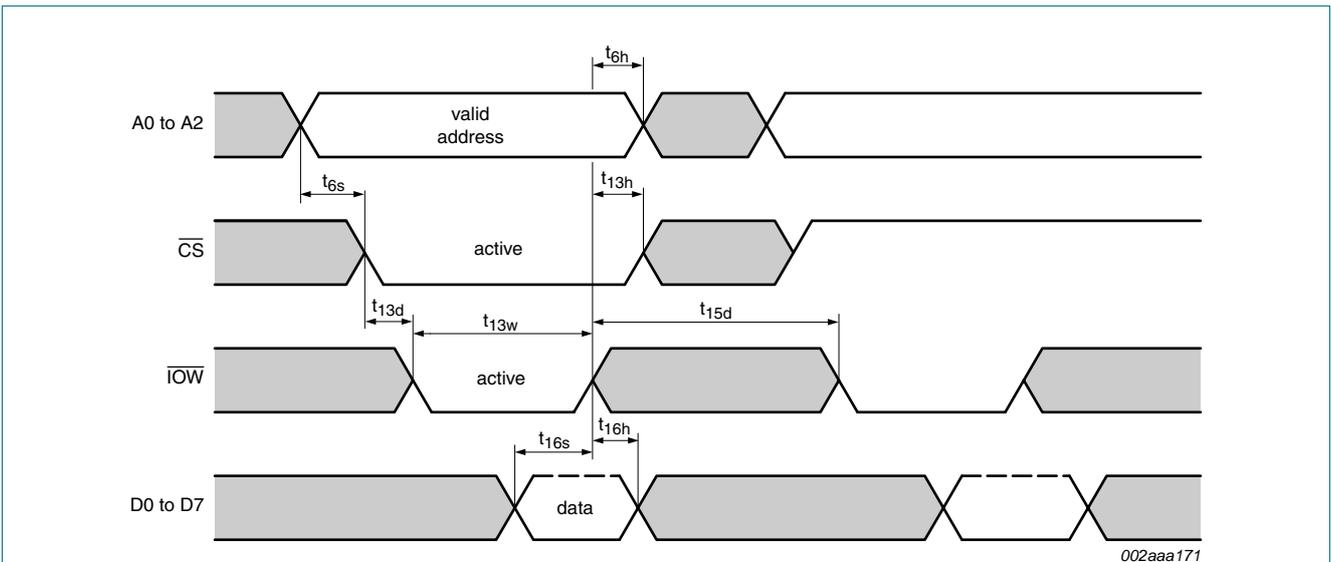
Fig 20. General write timing in 16 mode
