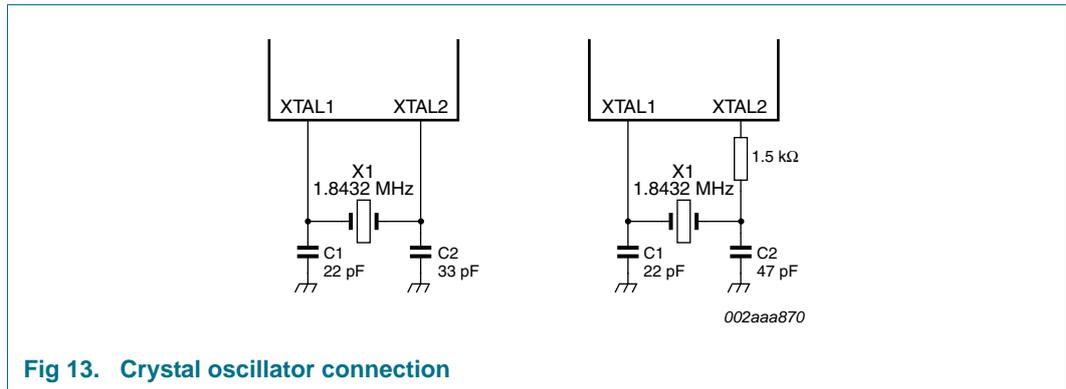
Fig 13. Crystal oscillator connection
