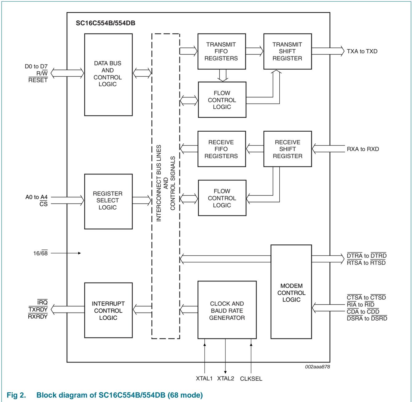
Fig 2. Block diagram of SC16C554B/554DB (68 mode)
