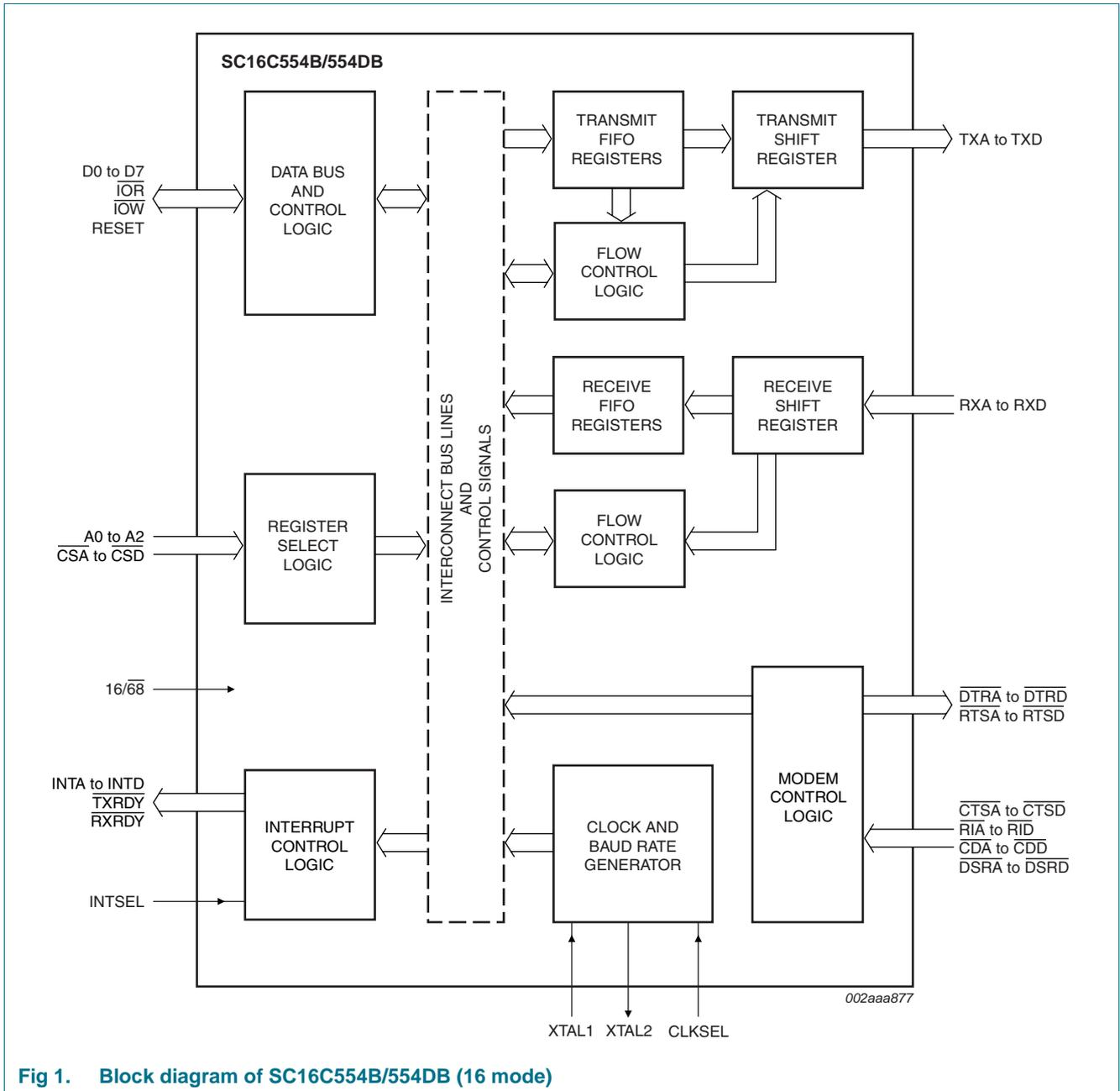
Fig 1. Block diagram of SC16C554B/554DB (16 mode)
