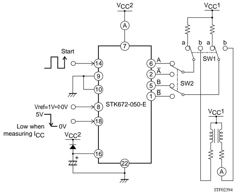
When measuring I<sub>oave</sub>: With SW1 set to 'a', V<sub>ref</sub> = 0.6V
