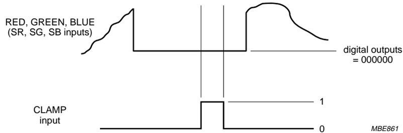
Fig.5 AC characteristics select signals; clamp and data.
