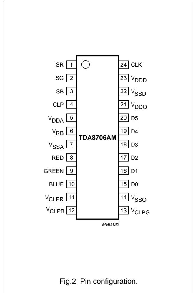
Fig.2 Pin configuration.
