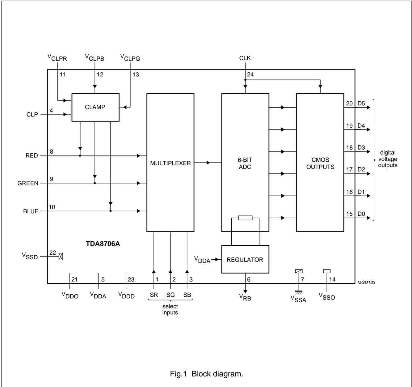
Fig.1 Block diagram.
