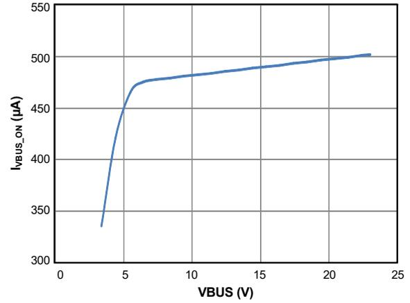
Figure 15. VBUS Quiescent Current vs. VBUS Voltage
