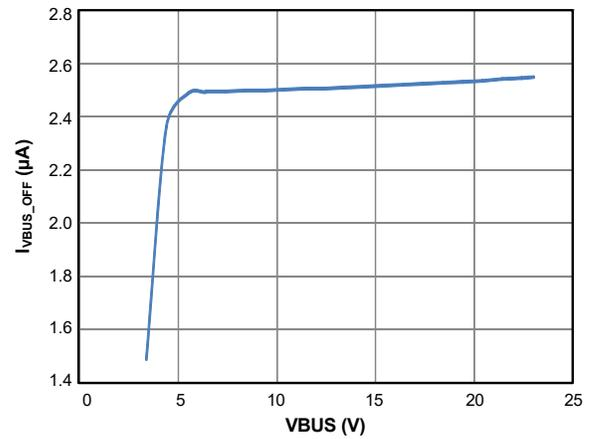
Figure 17. VBUS Shutdown Current vs. VBUS Voltage
