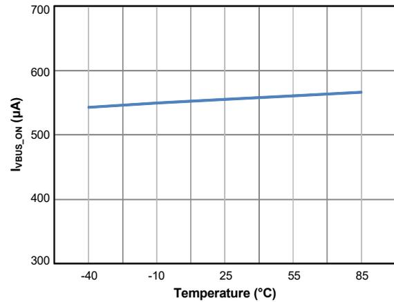
Figure 19. VBUS Quiescent Current vs. Temperature (VBUS=20V)
