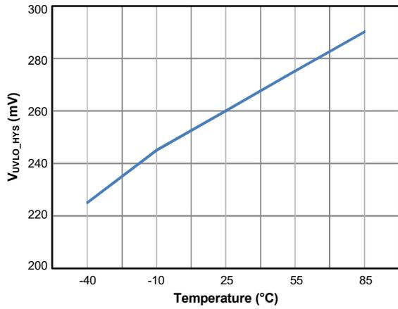
Figure 26. UVLO Hysteresis Voltage (VINT) vs. Temperature
