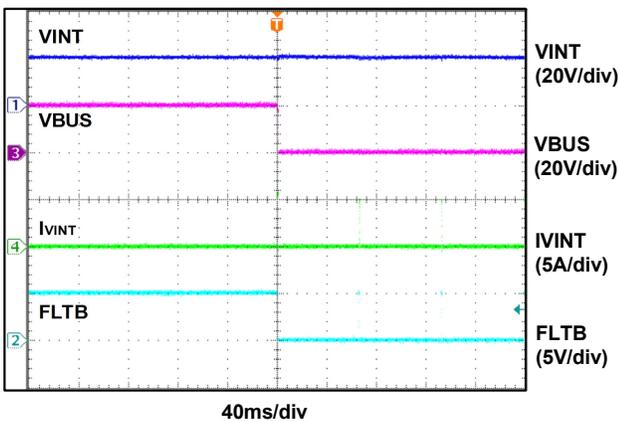
Figure 12. Short-Circuit Protection
