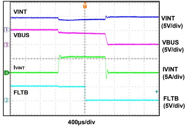
Figure 11. Over-Current Protection
