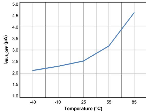
Figure 21. VBUS Shutdown Current vs. Temperature (VBUS=20V)
