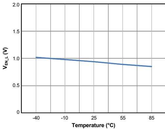
Figure 22. Enable Input Low Voltage vs. Temperature
