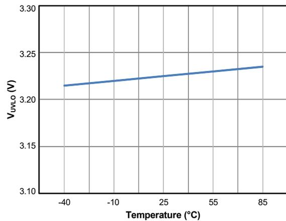
Figure 25. UVLO Rise Voltage (VBUS) vs. Temperature
