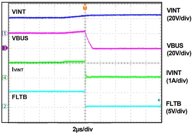
Figure 8. VINT OVP Operation with  $R_{OVP} = 20\text{k}\Omega$
