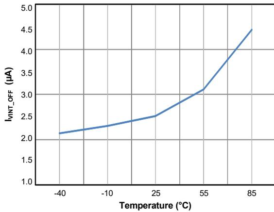
Figure 20. VINT Shutdown Current vs. Temperature (VINT=20V)
