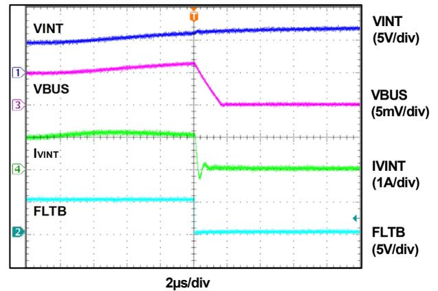
Figure 9. VINT OVP Operation with  $R_{OVP} = 180\text{k}\Omega$
