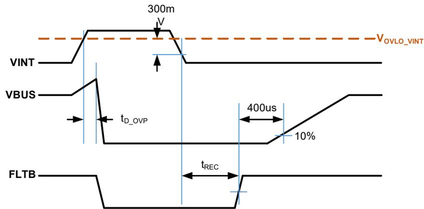
Figure 2. OVP Delay and Recovery Time for VINT OVP (AOZ1375DI-01)
