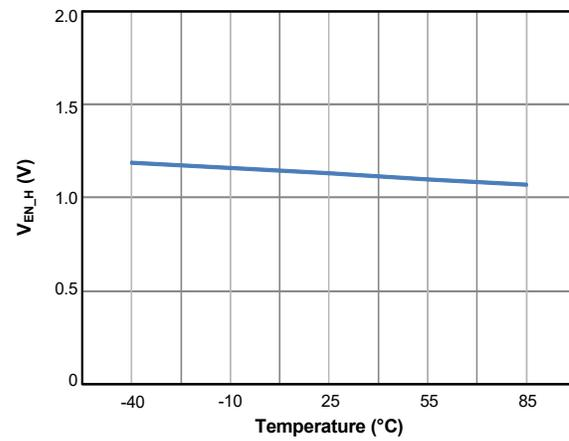
Figure 23. Enable Input High Voltage vs. Temperature
