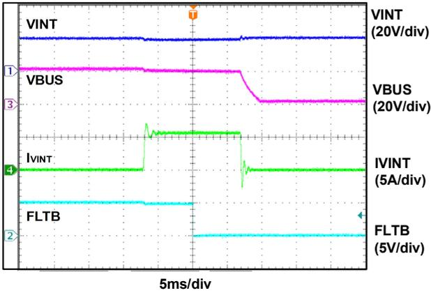
Figure 10. Over-Current Protection
