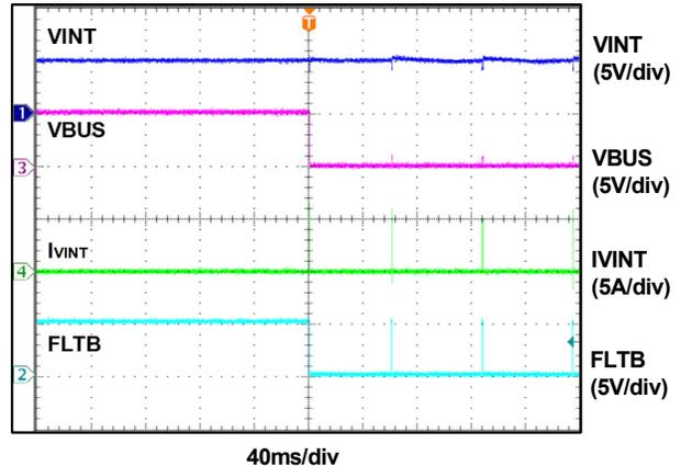
Figure 13. Short-Circuit Protection
