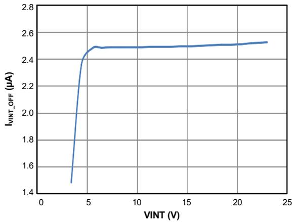
Figure 16. VINT Shutdown Current vs. VINT Voltage
