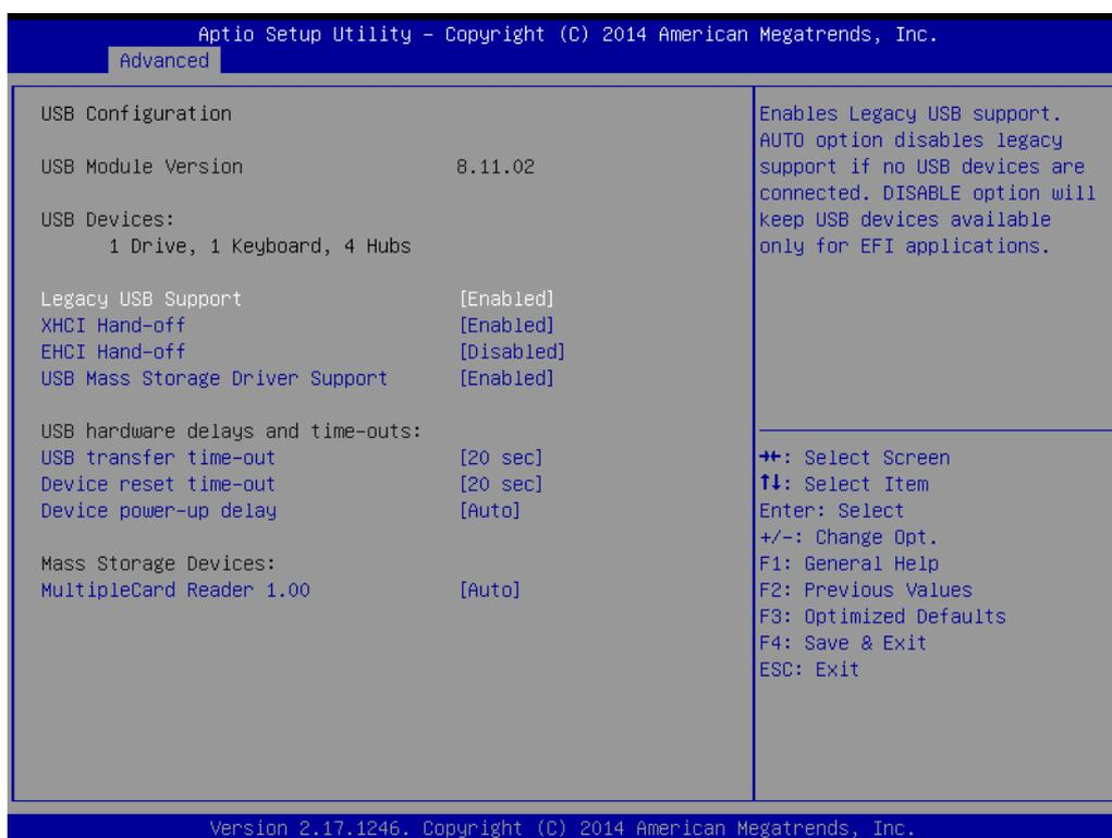
**Figure 3.9 USB Configuration setup screen**
