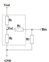
TRIM resistor connection (dashed line shows internal resistor network)
