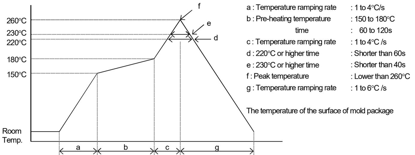
(NOTE1) Using reflow furnace with short wave infrared radiation heater such as halogen lamp
