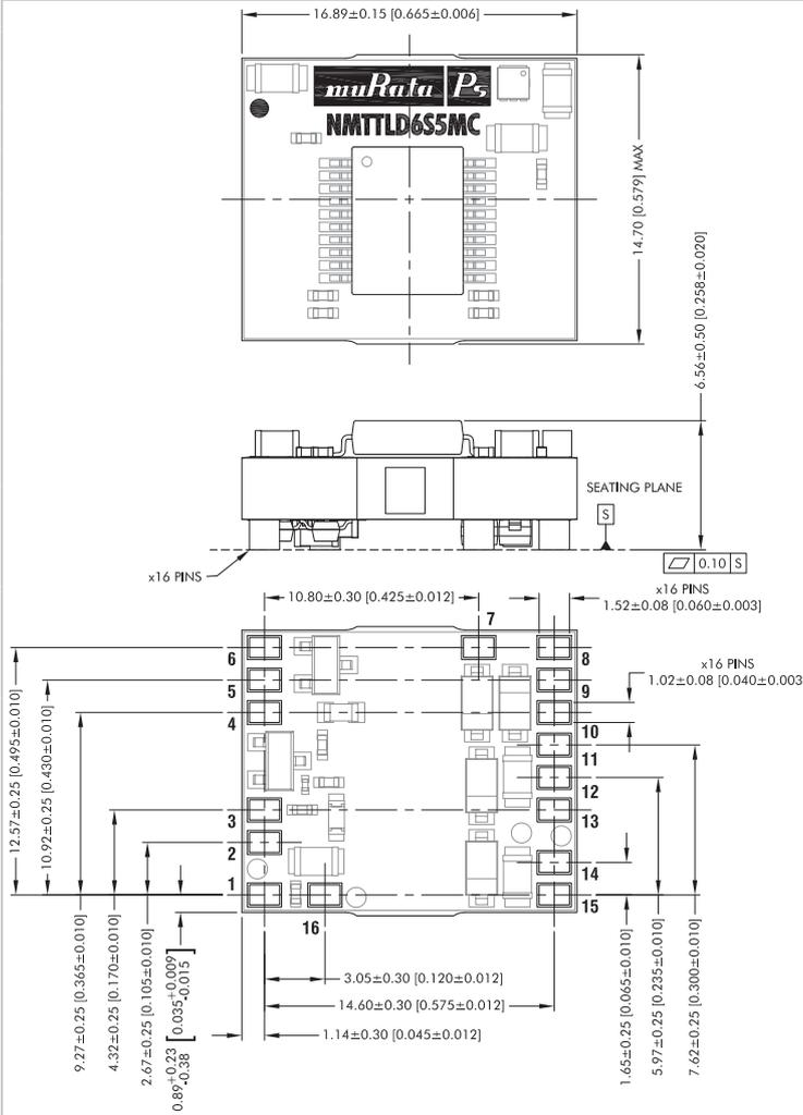
All dimensions in mm (inches). Controlling dimensions in mm.
