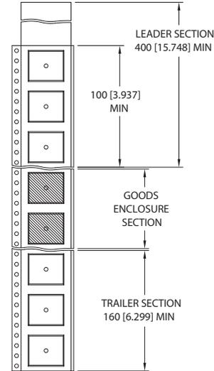
Carrier tape pockets shown are illustrative only - Refer to carrier tape diagram for actual pocket details.
