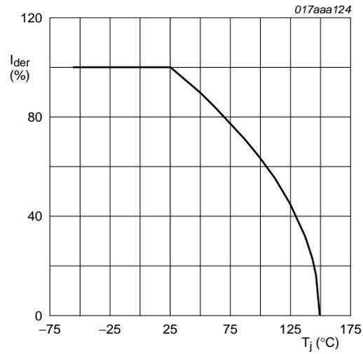
$$I_{der} = \frac{I_D}{I_{D(25^{\circ}\text{C})}} \times 100 \%$$
