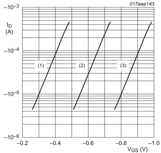
$T_j = 25\text{ }^\circ\text{C}; V_{DS} = -3\text{ V}$
