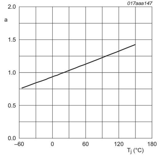
$$a = \frac{R_{DS(on)}}{R_{DS(on)@25^\circ\text{C}}}$$
