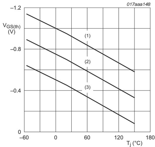
$I_D = -0.25\text{ mA}; V_{DS} = V_{GS}$
