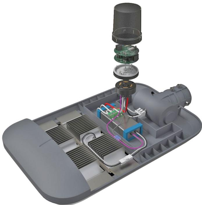
“TE CONNECTIVITY’S LUMAWISE ENDURANCE N INTERCONNECTS PROVIDE AN ANSI C136 COMPLIANT ELECTRICAL AND MECHANICAL INTERFACE CONNECTION FOR ROADWAY, STREET AND AREA LED LUMINAIRES AND CONTROLS. OUR IOT READY ECOSYSTEM, EMBEDDED WITH ELECTRONICS, SOFTWARE, SENSORS AND CONNECTIVITY ENABLES LUMINAIRES TO SERVE AS A LIGHTING SOURCE AND A COMMUNICATION DEVICE THAT COLLECTS AND EXCHANGES DATA.” ALEX HUNT III
