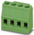
PCB terminal block, Nominal current: 24 A, Nom. voltage: 400 V, Pitch: 5 mm, Number of positions: 4, Connection method: Screw connection, Mounting: Soldering, Conductor/PCB connection direction: 0 °, Color: green, Article with lateral pin exit
