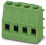
PCB terminal block, Nominal current: 24 A, Nom. voltage: 400 V, Pitch: 5 mm, Number of positions: 4, Connection method: Screw connection, Mounting: Soldering, Conductor/PCB connection direction: 0 °, Color: green, Article with lateral pin exit
