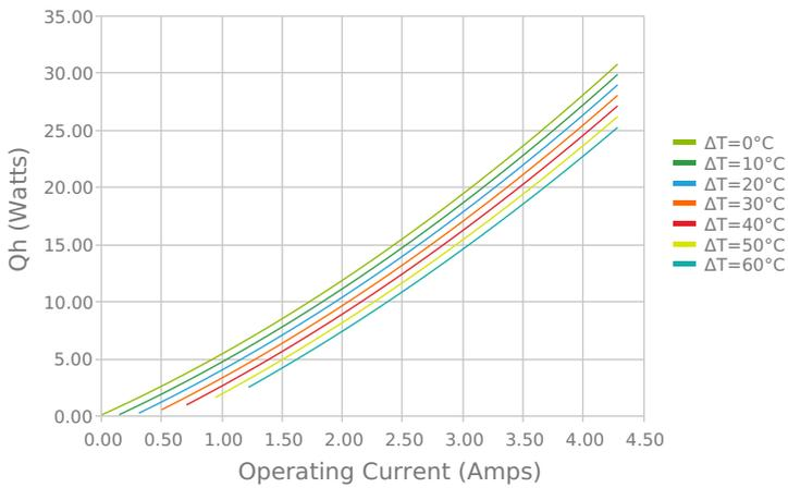
Total Heat Dissipated at Hot Side (Qh=Qc+Pin)
