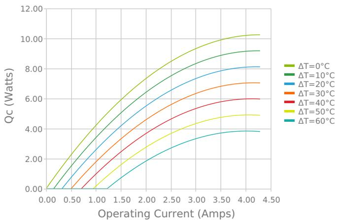
Heat Pumped at Cold Side
