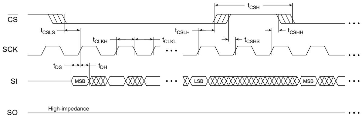
Figure 14-2. Serial Output Timing
