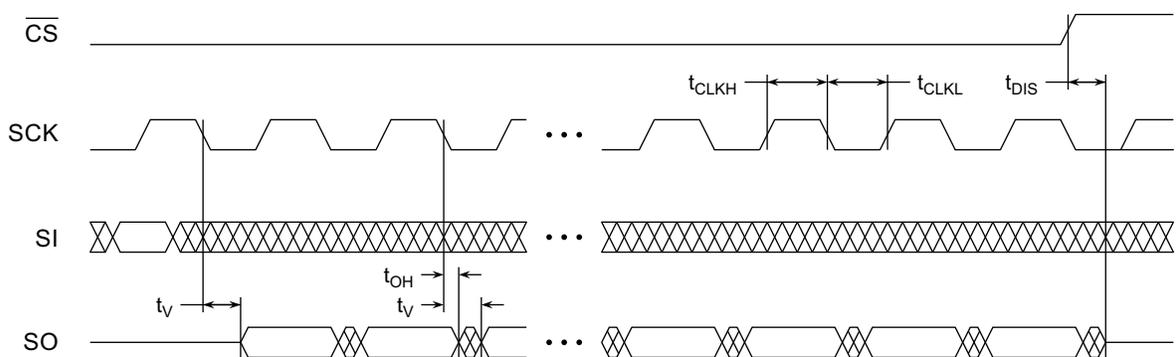
Figure 14-3.  $\overline{\text{WP}}$  Timing for Write Status Register Byte 1 Command When  $\text{SPRL} = 1$
