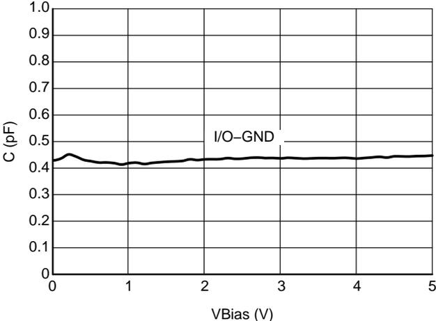
**Figure 2. CV Characteristics**
