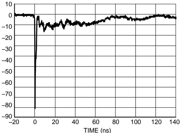
**Figure 4. IEC61000-4-2 -8 kV Contact ESD Clamping Voltage**
