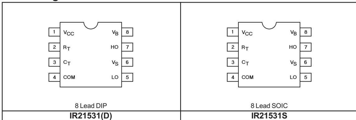
NOTE: The IR21531D is offered in 8 lead DIP only.
