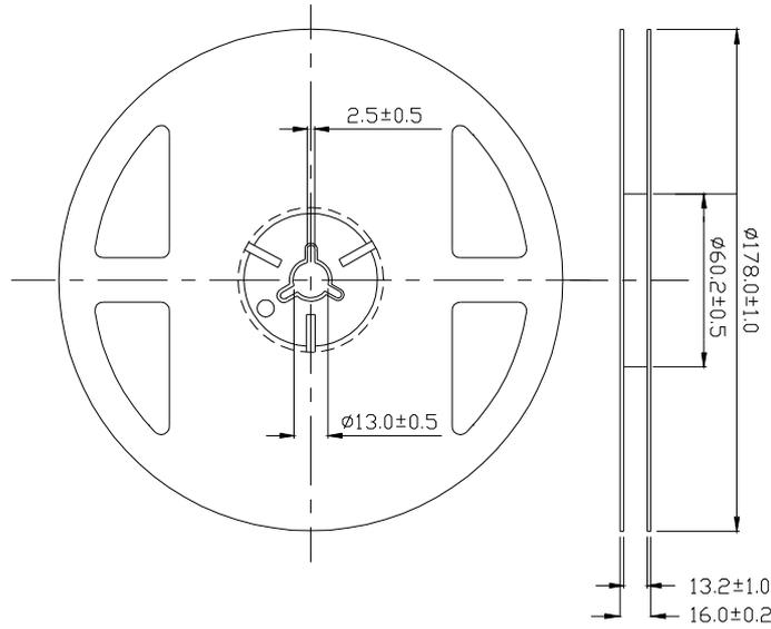
Note: The tolerances unless mentioned are  $\pm 0.1$ , unit=mm.
