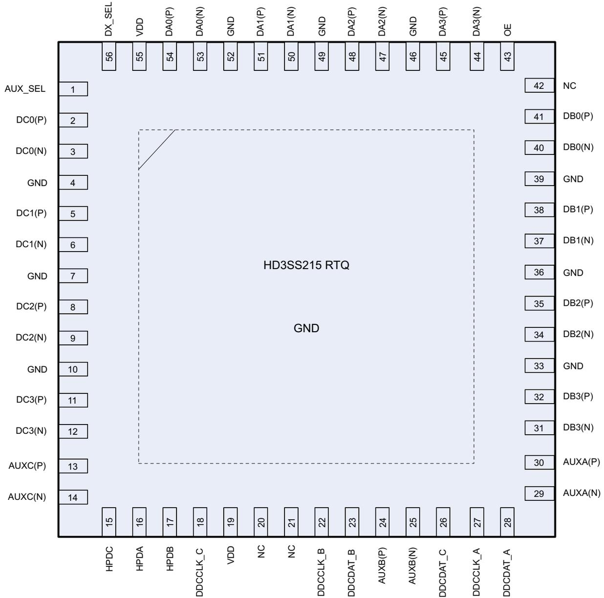
**Figure 6-2. 56-Pin QFN RTQ Package (Top View)**
