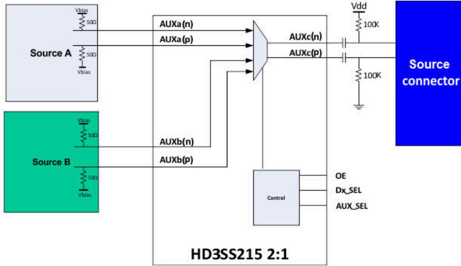
Figure 9-2. HD3SS215 AUX Channel in 2:1 DisplayPort Application
