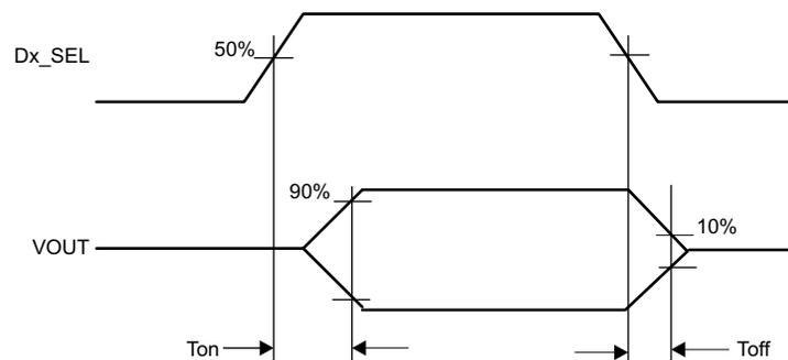
Figure 7-1. Select to Switch t<sub>on</sub> and t<sub>off</sub>
