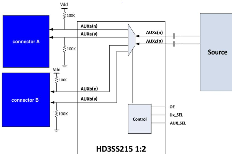
Figure 9-3. HD3SS215 AUX Channel in 1:2 DisplayPort Application
