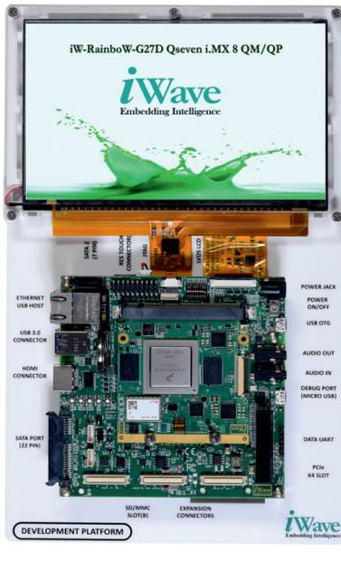
The i.MX 8 QM/QP (Quad Max/Quad Plus) Qseven Development platform combines the NXP i.MX 8 QM/QP application processor based Qseven SOM and iWave's Generic Qseven Carrier Card to offer maximum performance with higher efficiency for complex consumer, medical and industrial embedded computing applications. The board is highly packed with all necessary onboard connectors to validate i.MX 8 QM/QP SoC features to the fullest.
