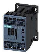
Traction contactor, AC-3 16 A, 7.5 kW / 400 V 1 NC, 24-34 V DC, 0.7-1.25\*Us with integrated varistor Size S00, Spring-type terminals suitable for PLC outputs
