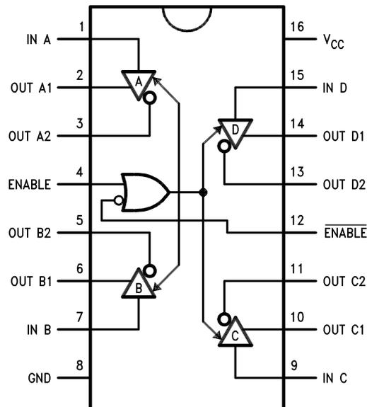
**Figure 1. 16-Lead CDIP Package- Top View**
