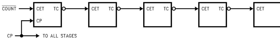
Figure 1. Multistage Counter with Ripple Carry
