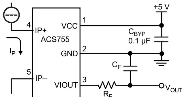
Application 1. The ACS755 outputs an analog signal,  $V_{OUT}$ , that varies linearly with the unidirectional DC primary sensed current,  $I_P$ , within the range specified.  $C_F$  is recommended for noise management, with values that depend on the application.
