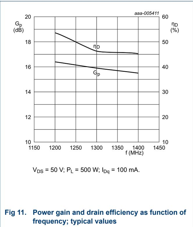
7.4.3 Performance curves measured with  $\delta = 10 \%$ ,  $t_p = 300 \mu\text{s}$  and  $f = 1300 \text{ MHz}$
