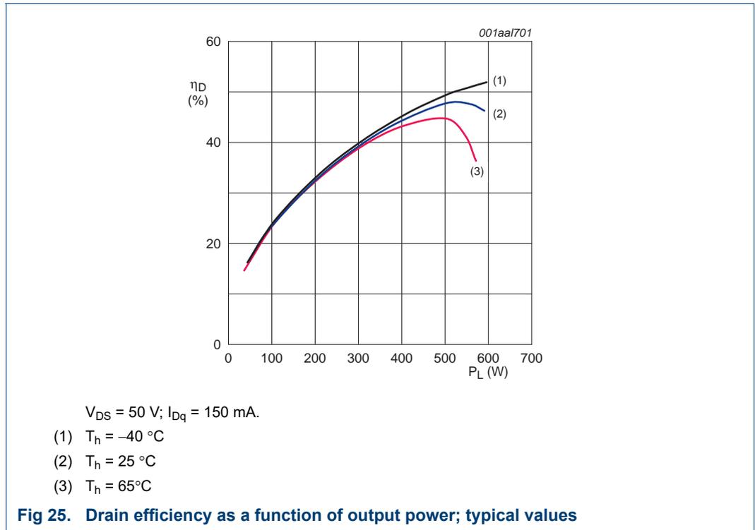
**7.4.7 Performance curves measured with  $\delta = 10 \%$ ,  $t_p = 1 \text{ ms}$  and  $T_h = 25 \text{ }^\circ\text{C}$**
