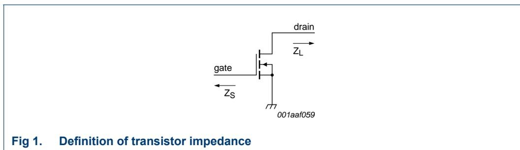
**Fig 1. Definition of transistor impedance**
