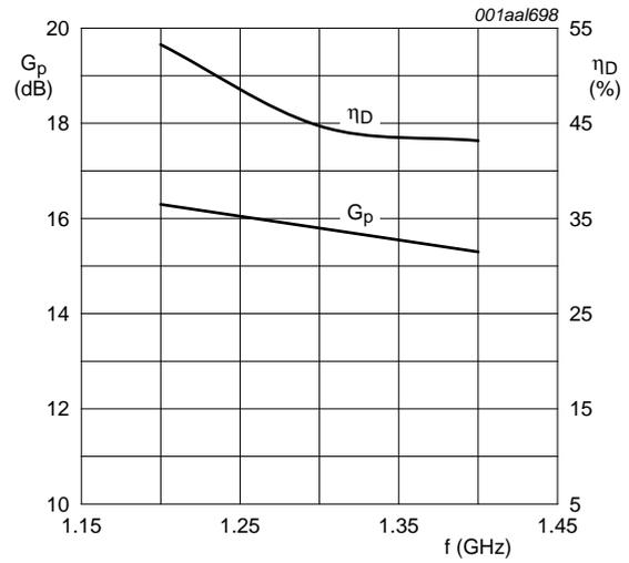
$V_{DS} = 50 \text{ V}; I_{Dq} = 150 \text{ mA}.$
