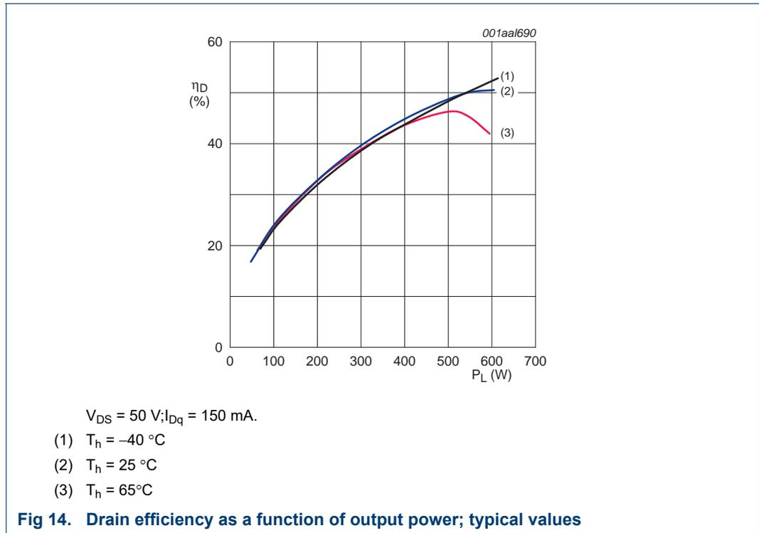
**7.4.4 Performance curves measured with  $\delta = 20\%$ ,  $t_p = 500\ \mu\text{s}$  and  $T_h = 25\text{ }^\circ\text{C}$**
