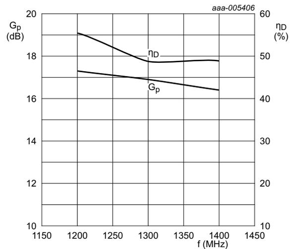
$V_{DS} = 50 V$ ;  $P_L = 500 W$ ;  $I_{Dq} = 150 mA$ .
