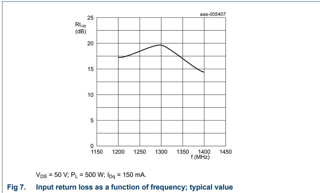
**7.4.2 Performance curves measured with  $\delta = 10 \%$ ,  $t_p = 300 \mu\text{s}$  and  $T_h = 65 \text{ }^\circ\text{C}$**
