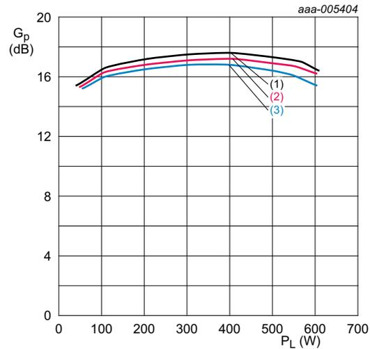
$V_{DS} = 50 V$ ;  $I_{Dq} = 150 mA$ .
