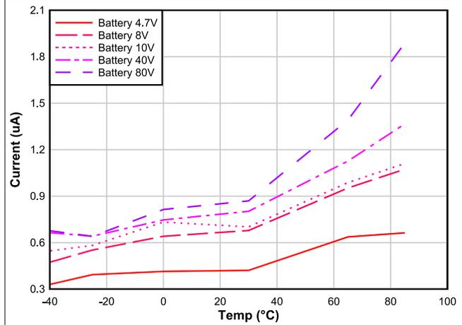
Figure 7-29. BAT Current in SHUTDOWN Mode vs. Temperature
