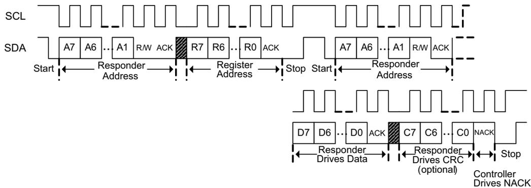
**Figure 14-3. I<sup>2</sup>C Read Without Repeated Start**
