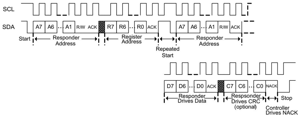
Figure 14-2. I<sup>2</sup>C Read with Repeated Start
