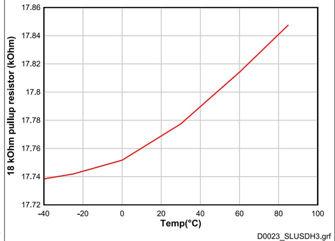
**Figure 7-21. Thermistor Pullup Resistance vs. Temperature (18-kΩ Setting)**
