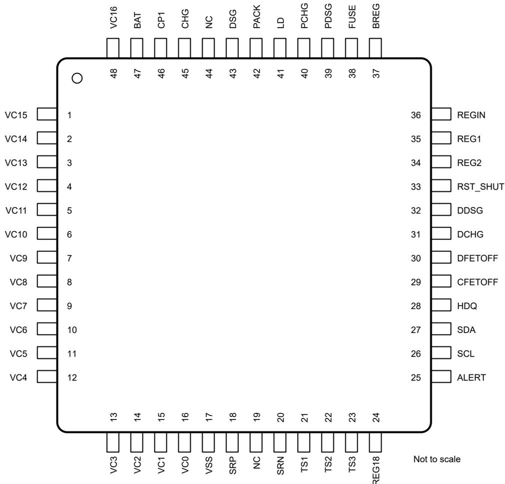
Table 6-1. BQ76952 TQFP Package (PFB) Pin Functions
