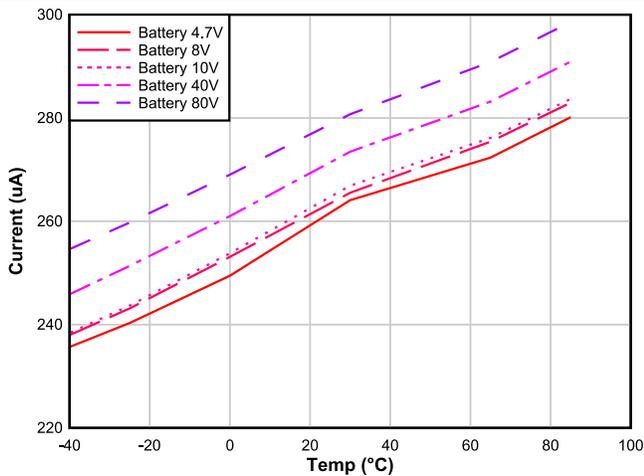
Figure 7-28. BAT Current in NORMAL Mode vs. Temperature
