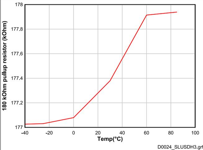
**Figure 7-22. Thermistor Pullup Resistance vs. Temperature (180-kΩ Setting)**
