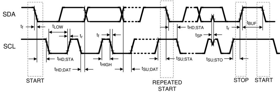
**Figure 7-1. I<sup>2</sup>C Communications Interface Timing**
