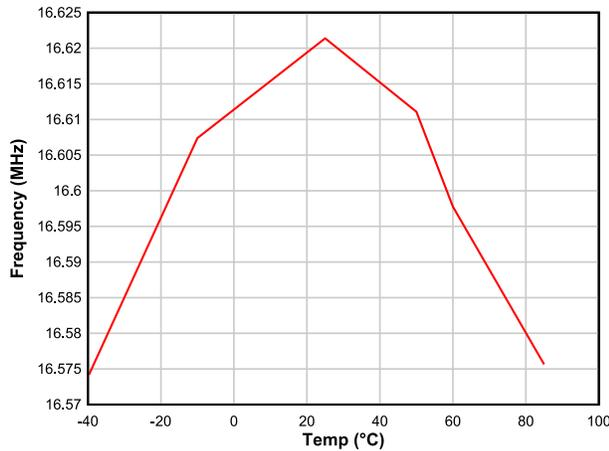
**Figure 7-14. High Frequency Oscillator (HFO) Accuracy vs. Temperature**
