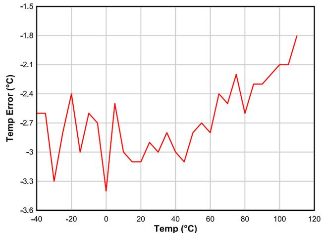
Measurements taken using Semitec 103-AT thermistor, default temperature polynomial, and 18-k $\Omega$  internal pullup resistor.
