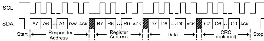
Figure 14-1. I<sup>2</sup>C Write
