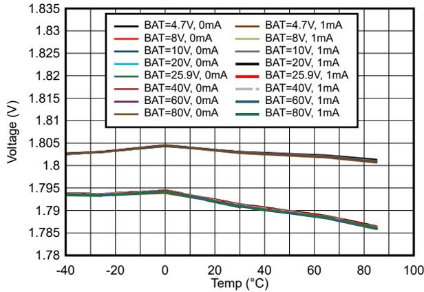
Figure 7-26. REG18 Voltage vs. Temperature, Across BAT Levels
