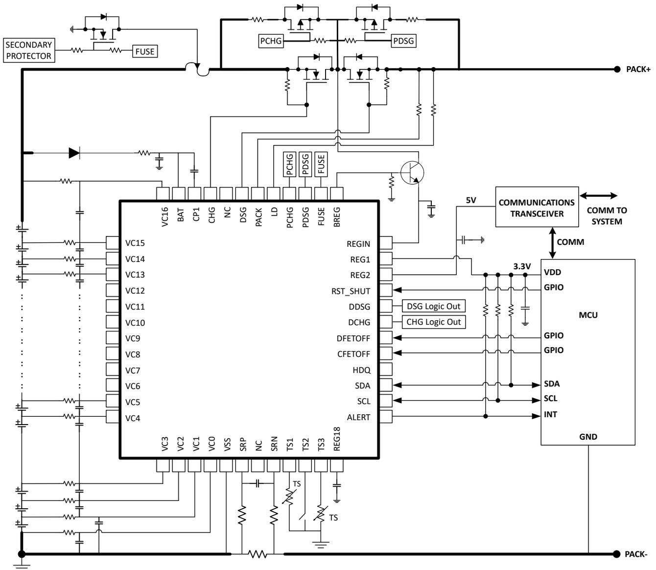
**Figure 16-1. BQ76952 16-Series Cell Typical Implementation (Simplified Schematic)**
