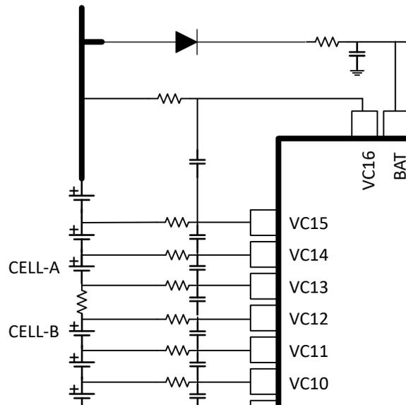
**Figure 10-1. Using Cell Input Pins for Interconnect Measurement**
