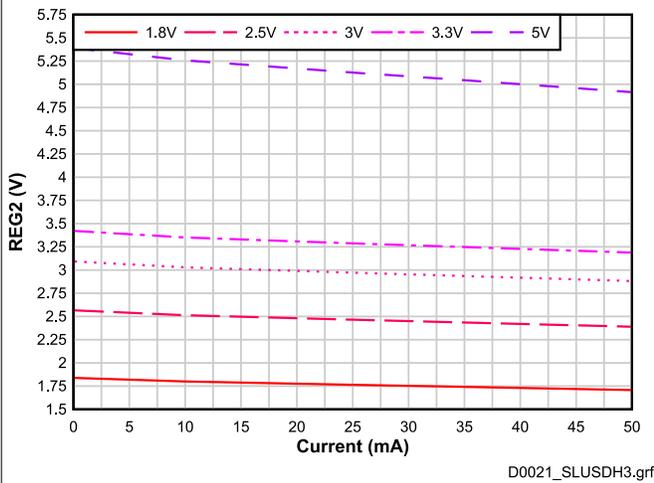
**Figure 7-20. REG2 Voltage vs. Load at 25°C**
