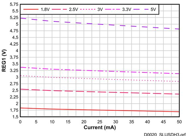
**Figure 7-19. REG1 Voltage vs. Load at 25°C**
