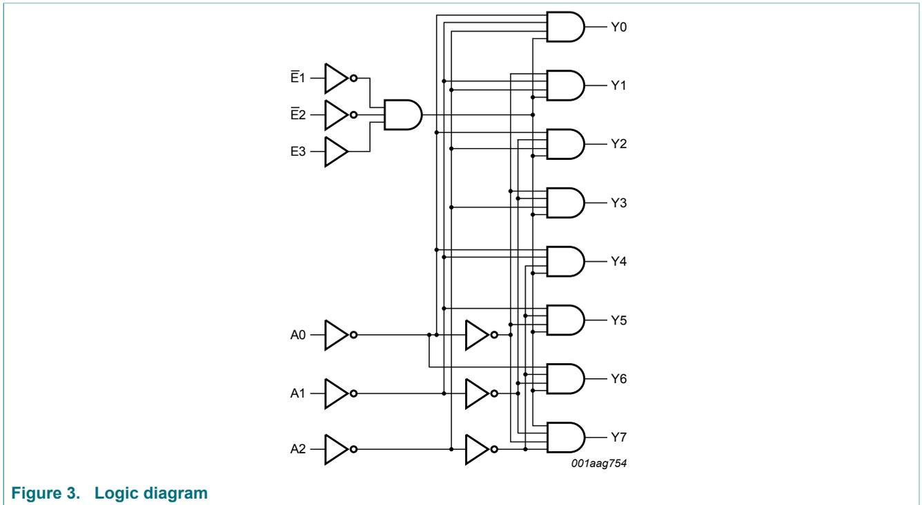
Figure 3. Logic diagram
