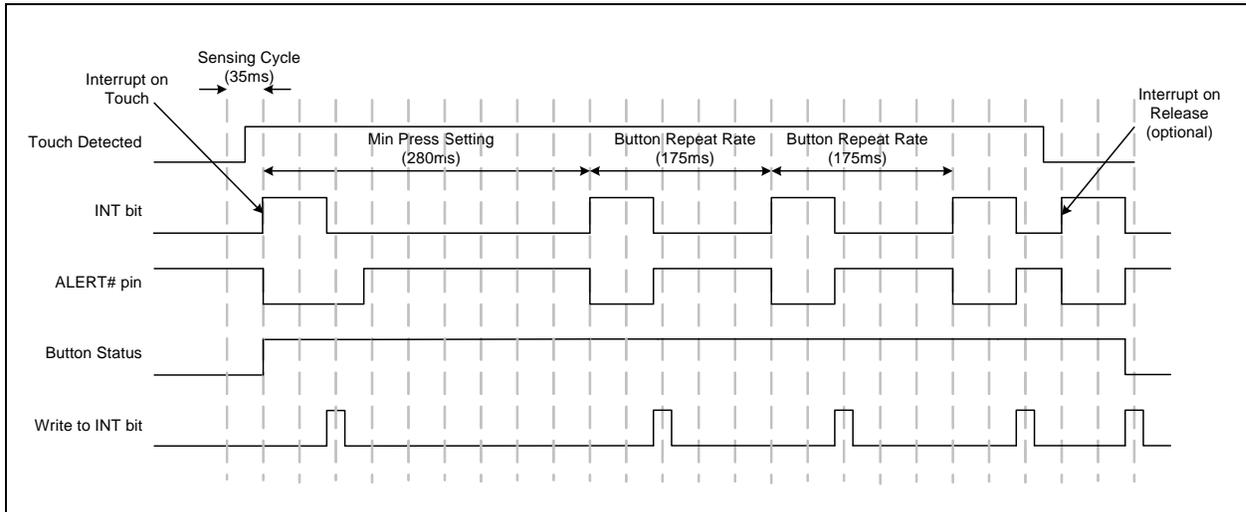
**FIGURE 4-5: SENSOR INTERRUPT BEHAVIOR - NO REPEAT RATE ENABLED**
