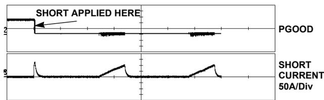
**HICUP MODE. SUPPLY POWERED BY ATX SUPPLY**
