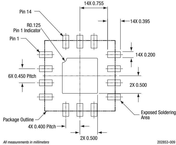
**Figure 9. SKY13526-485LF PCB Layout Footprint (Top View)**
