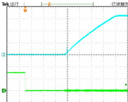
**Figure 4:** Turn-on transient at full rated load current (4 ms/div).  $V_{in}=48V$ . Top Trace:  $V_{out}$ , 1.0V/div; Bottom Trace: ON/OFF input, 2V/div
