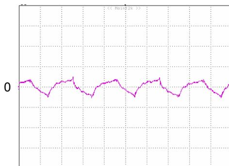
**Figure 14:** Output voltage ripple at nominal input voltage and rated full load current (100 mV/div, 1µs/div)
