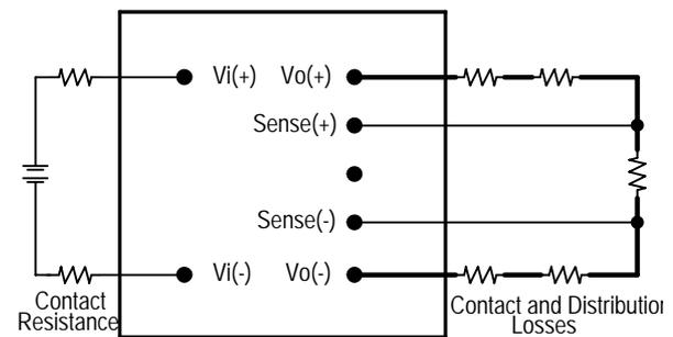
Figure 16: Effective circuit configuration for remote sense operation
