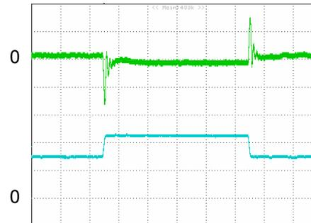
**Figure 9:** Output voltage response to step-change in load current (75%-50%-75% of  $I_{o, max}$ ;  $di/dt = 1.0A/\mu s$ ). Load cap: 10 $\mu F$  tantalum capacitor and 1 $\mu F$  ceramic capacitor. Top Trace:  $V_{out}$  (100mV/div, 200us/div), Bottom Trace:  $I_{out}$  (20A/div). Scope measurement should be made using a BNC cable (length shorter than 20 inches). Position the load between 51 mm to 76 mm (2 inches to 3 inches) from the module
