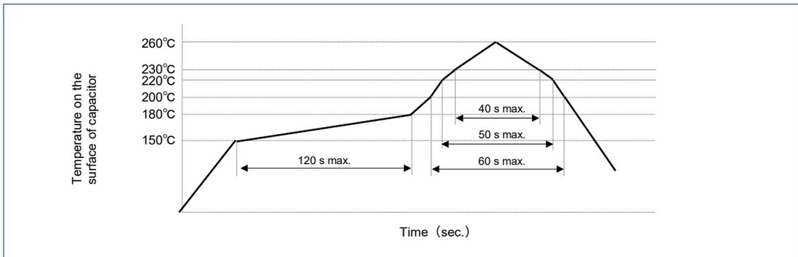
◇ **Flow soldering (Radial lead type)**
