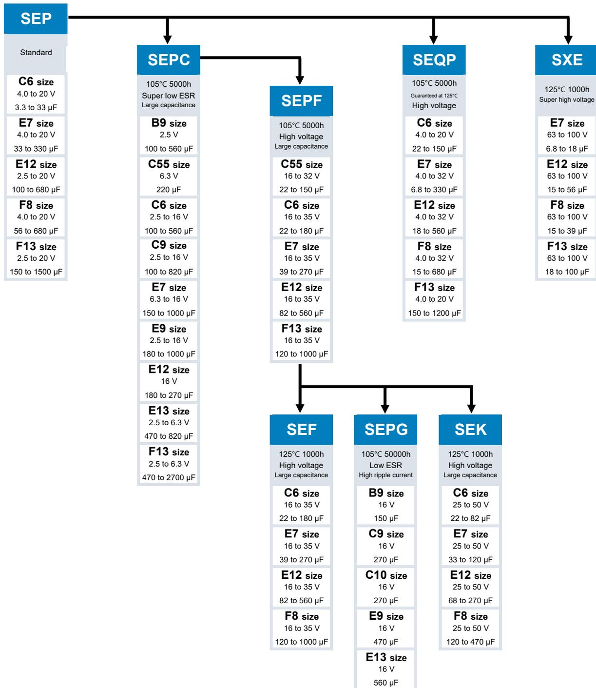
**Voltage - Capacitance table (SMD type) (Vol. : 2.0 to 16 V / Cap. : 3.3 to 33  $\mu$ F)**
