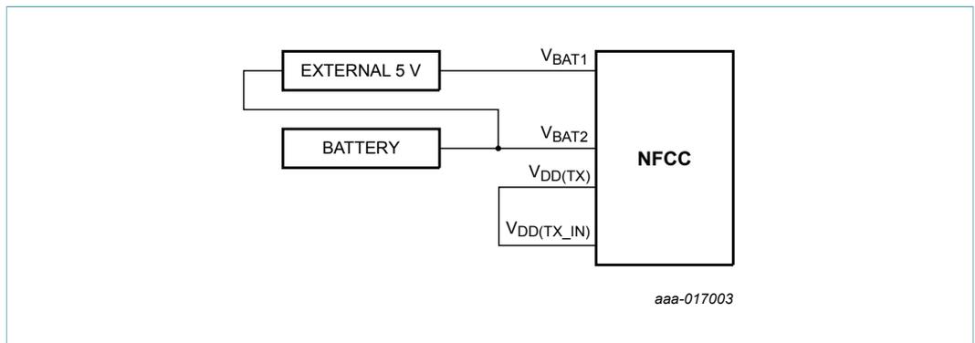
Fig 15.  $V_{BAT1} = 5$  V,  $V_{BAT2}$  between 2.3 V and 5.5 V
