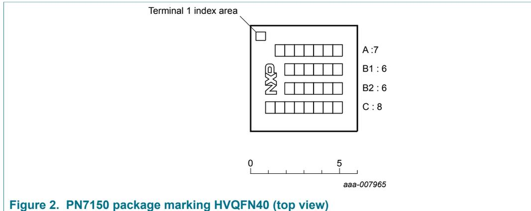
Figure 2. PN7150 package marking HVQFN40 (top view)
