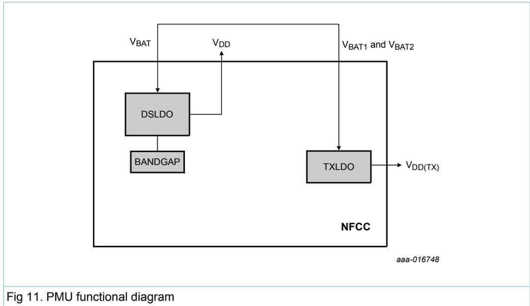
Fig 11. PMU functional diagram
