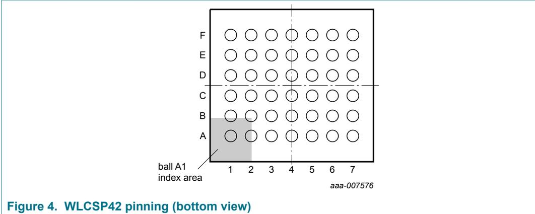
Figure 4. WLCSP42 pinning (bottom view)
