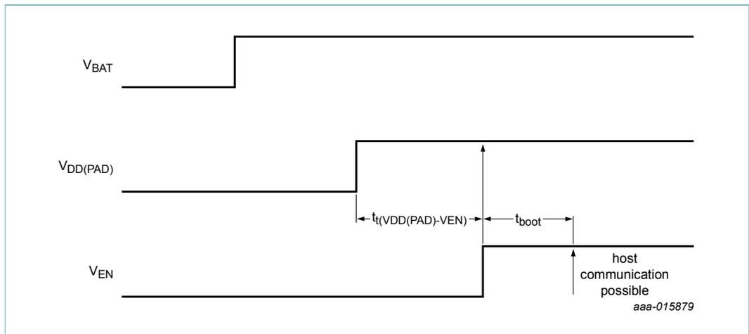
Fig 19. V<sub>BAT</sub> is set up before V<sub>DD(PAD)</sub>
