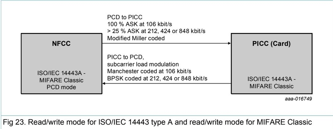
Fig 23. Read/write mode for ISO/IEC 14443 type A and read/write mode for MIFARE Classic
