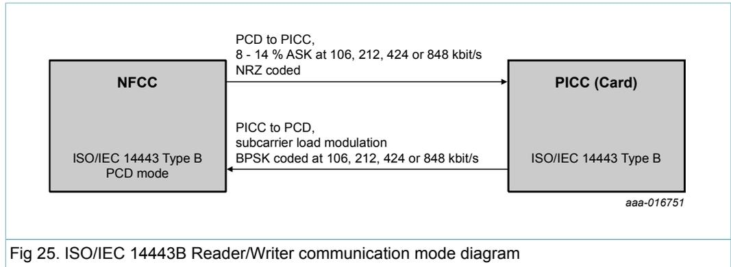
Fig 25. ISO/IEC 14443B Reader/Writer communication mode diagram
