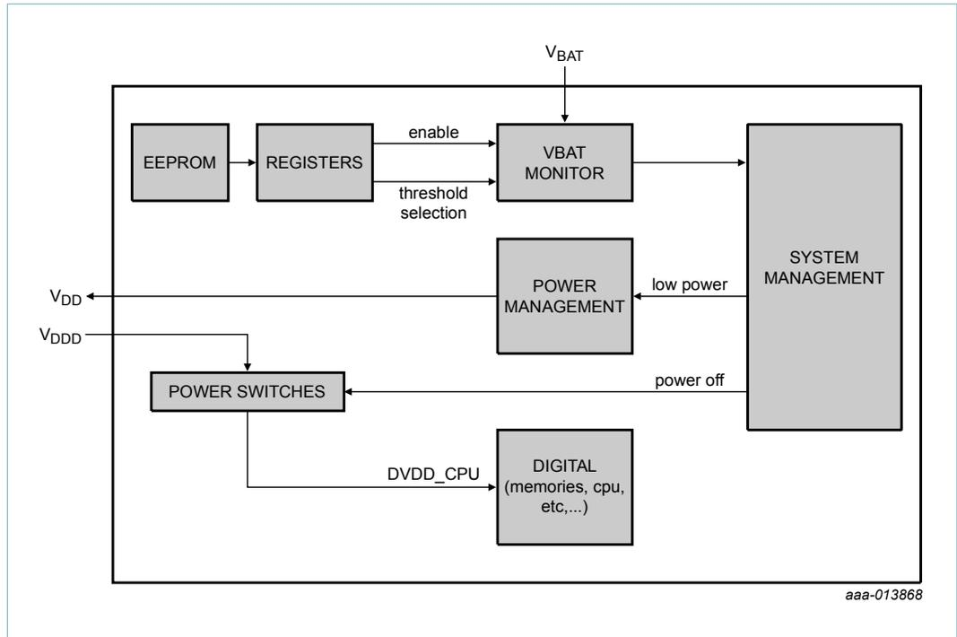
Fig 17. Battery voltage monitor principle
