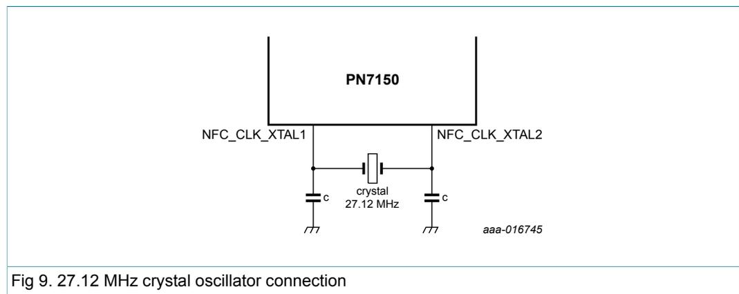
Fig 9. 27.12 MHz crystal oscillator connection
