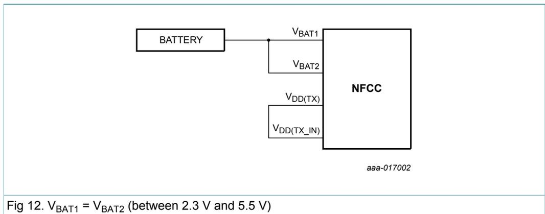
Fig 12. V<sub>BAT1</sub> = V<sub>BAT2</sub> (between 2.3 V and 5.5 V)
