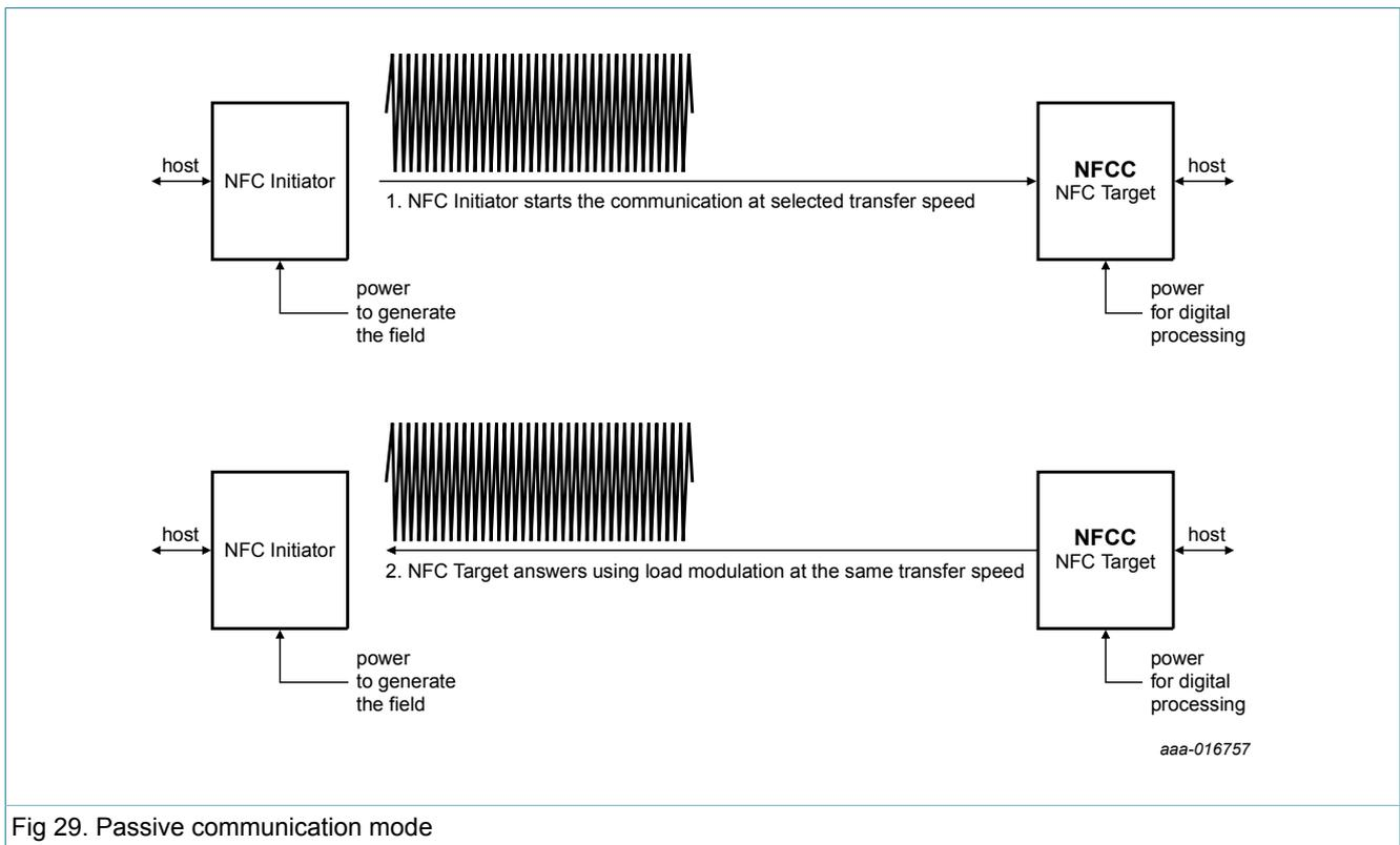
Fig 29. Passive communication mode
