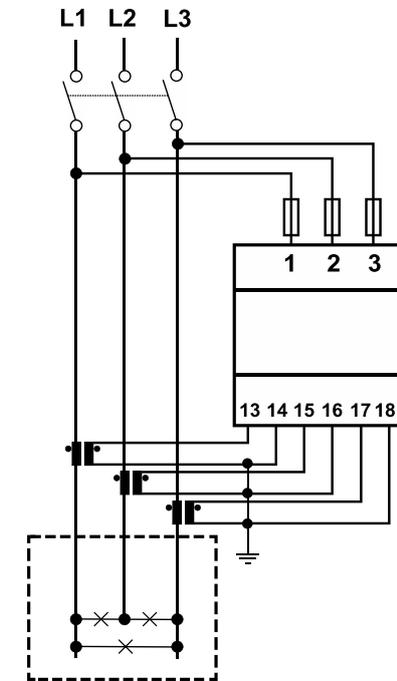
**Fig. 4** Three-phase without neutral (3-wire)
