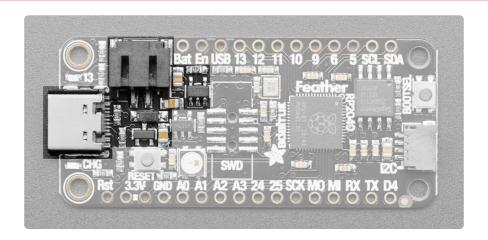
The above shows the USB-C jack (left), LiPoly JST jack (top left), as well as the changeover diode (just to the right of the JST jack) and the LiPoly charging circuitry (to the right of the JST jack).
