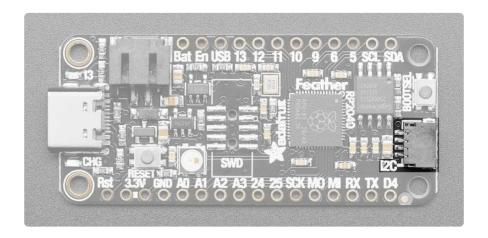
The Feather RP2040 comes with a built in STEMMA QT connector! This means you can connect up all sorts of I2C sensors and breakouts (), no soldering required! This connector uses the SCL and SDA pins for I2C, which ends up being the RP2040's I2C1 peripheral. In CircuitPython, you can use the STEMMA connector with board.SCL and board.SDA, or board.STEMMA\_I2C(). In Arduino it is Wirel.
