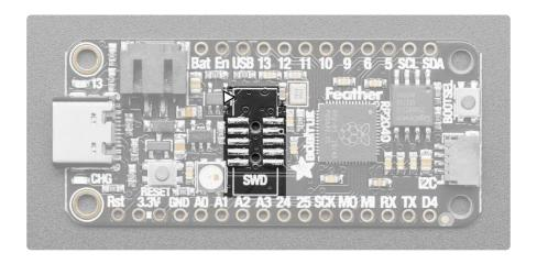
For advanced debugging or to reprogram your Feather RP2040, there is a footprint to solder a 2\*5 pin 0.05" standard SWD header on the board. The image above shows the "pin 1" location by marking it with a triangle. This orientation places the connector key facing towards the end of the board where the USB connector is. This allows you to use something like a <a href="Segger J-Link">Segger J-Link</a> () and a <a href="1.27mm">1.27mm</a> SWD cable</a> () to connect from your PC to the Feather.
