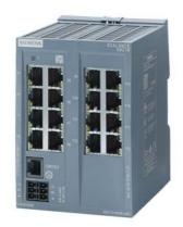
SCALANCE XB216 managed Layer 2 IE switch, 16X 10/100 Mbit/s RJ45 ports, 1x console port, diagnostics LED redundant power supply IEC 62443-4-2 certified; temperature range 0 °C to +60 °C; DIN-rail mounting, PROFINET IO device Ethernet/IP certificate, default PROFINET.
