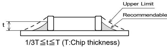
Accordingly increasing the solder volume, the mechanical stress to product is also increased. Exceeding solder volume may cause the failure of mechanical or electrical performance.
