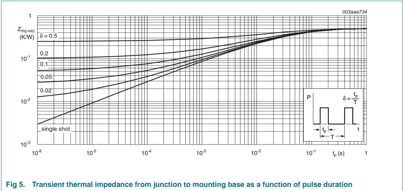
Fig 5. Transient thermal impedance from junction to mounting base as a function of pulse duration
