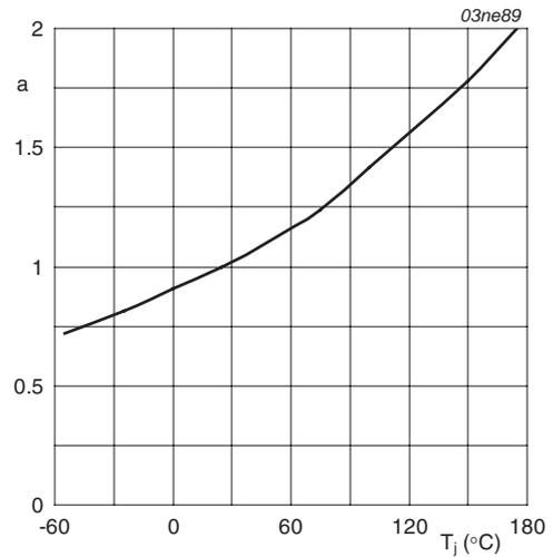
$$a = \frac{R_{DSon}}{R_{DSon(25^\circ\text{C})}}$$
