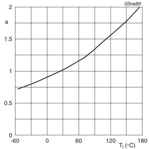
$$a = \frac{R_{DSon}}{R_{DSon(25^\circ\text{C})}}$$
