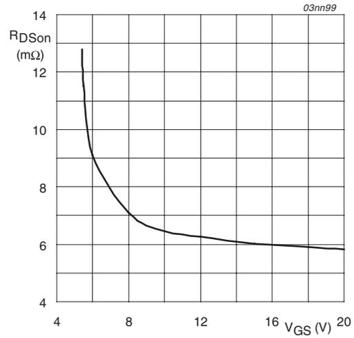
$T_j = 25^\circ\text{C}; I_D = 50\text{A}$
